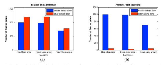
Fig. 3. The statistical chart for the simulation environment: (a) number of detected feature points and (b) number of matched features points
