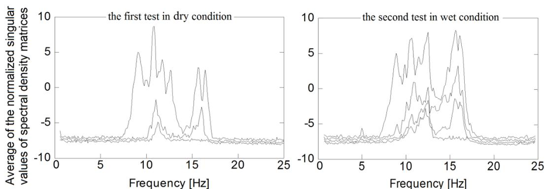
Fig. 5 The frequency domain decomposition plots derived from the tests on the bridge on two different condition of the riverbed
