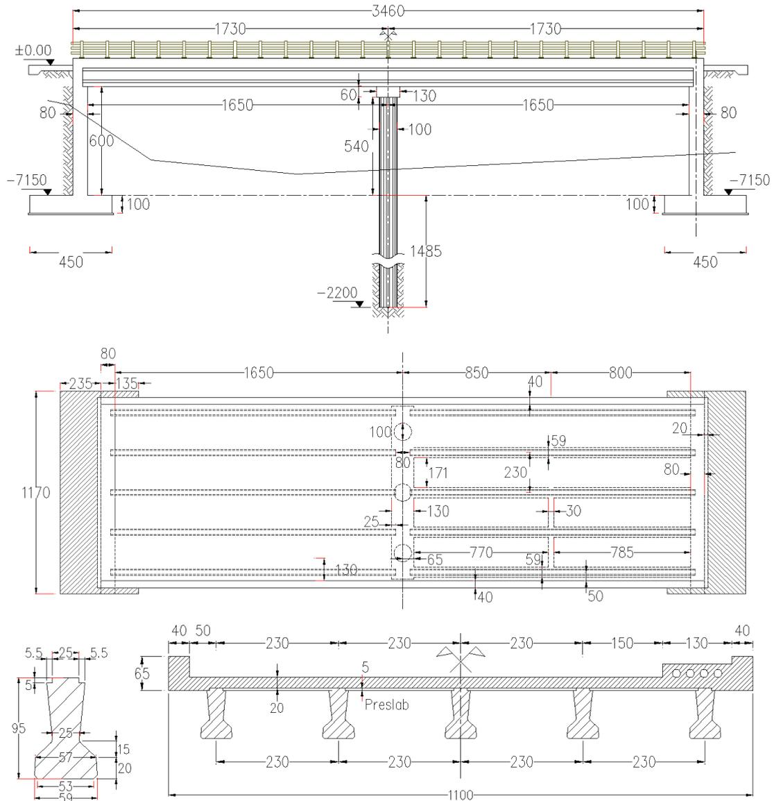
Fig. 2 Geometrical dimensions and cross sections of the bridge (Dimensions are in cm)
