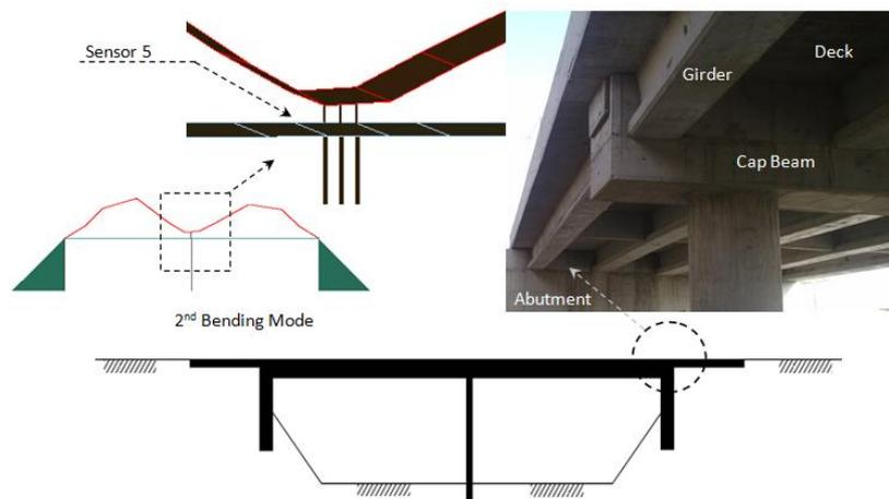
Fig. 8 Rigidity of the superstructure-pier connection
