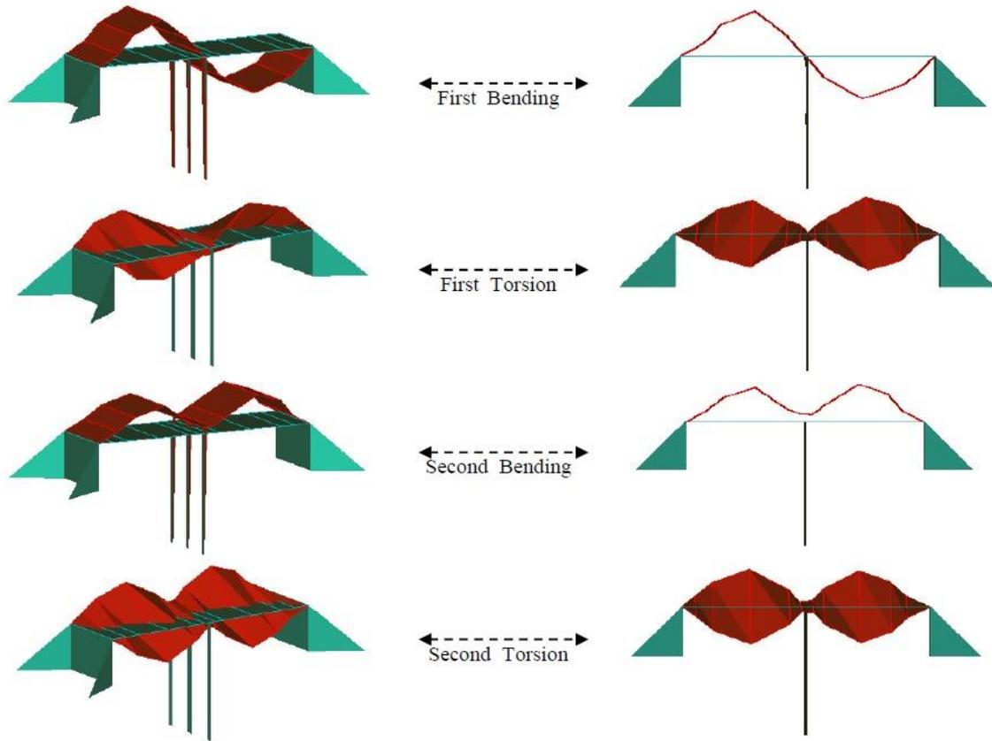
Fig. 6 Mode shapes identified from the first test carried out on the bridge
