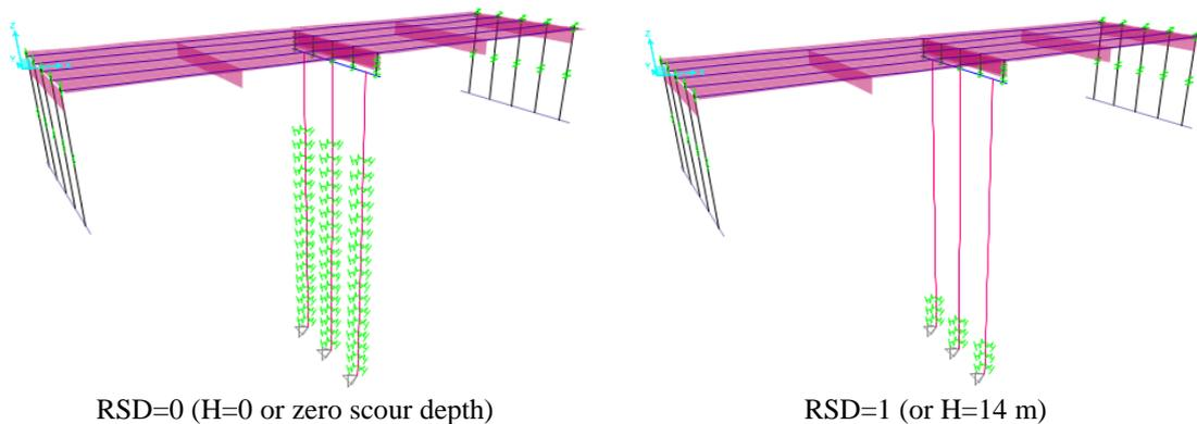
Fig. 12 Two FE models of the bridge, representing the RSD=0 and 1
