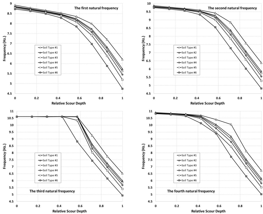
Fig. 13 Variation of the first four natural frequencies of the bridge with respect to the RSD for different sub-soils
