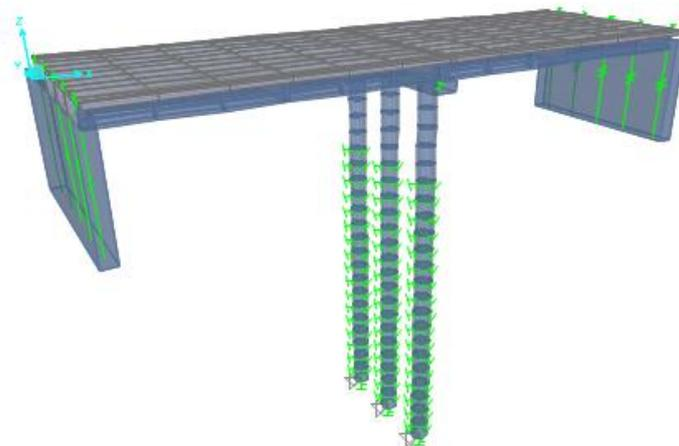
Fig. 9 The FE model of the bridge
