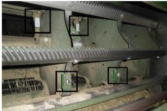
Fig. 11 the locations of applying mass on the thresher
