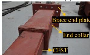
(b) Brace ends construction detail
