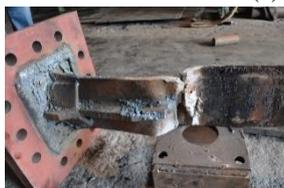
(b) Local buckling and rupture at one end
