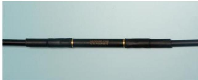
Fig. 8 FBG-based temperature sensor
