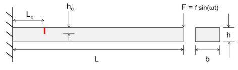
Fig. 1 Cantilever beam with a breathing crack
