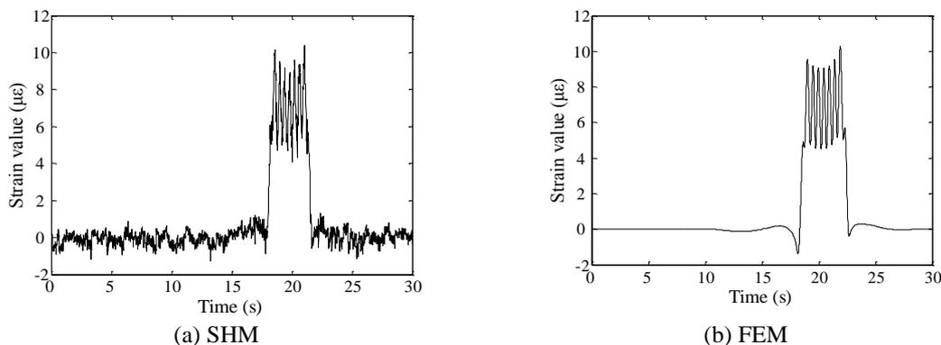
Fig. 5 Time history curve of  $Y_1$  strain value of single drive in case 6
