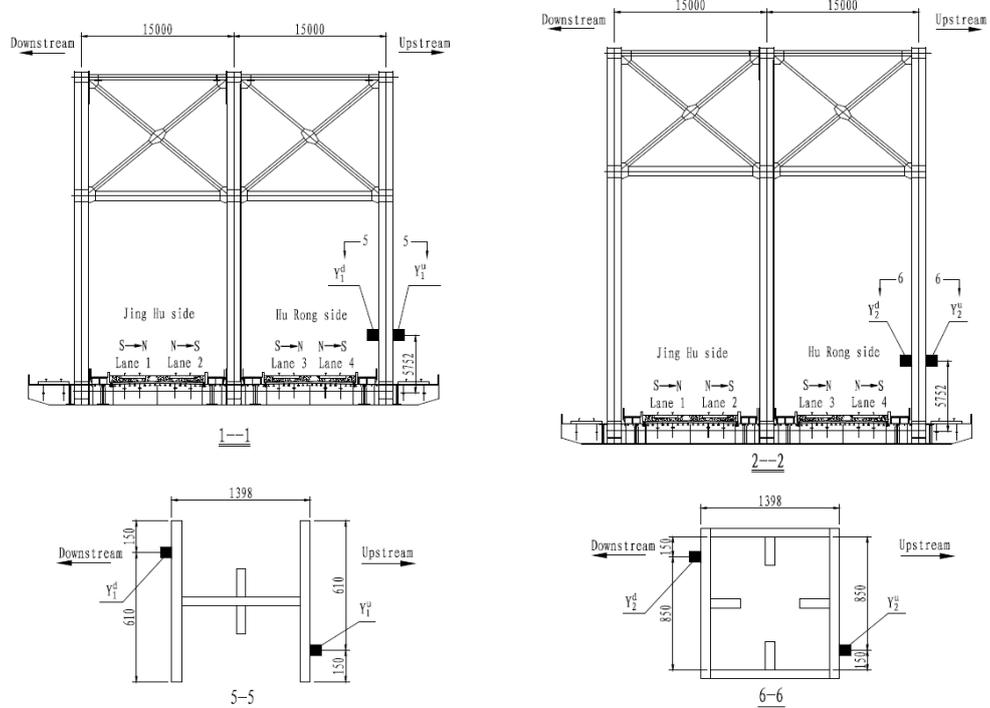
(a) 1-1 cross-section of steel truss arch
