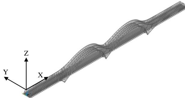
Fig. 3 Three-dimensional FEM of Nanjing DSG Bridge
