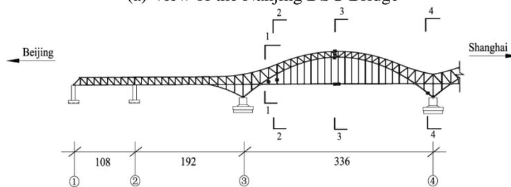
(b) Elevation drawing of half part bridge (Unit: m)
