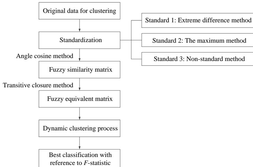
Fig. 4 Flow chart of transitive closure fuzzy clustering analysis method
