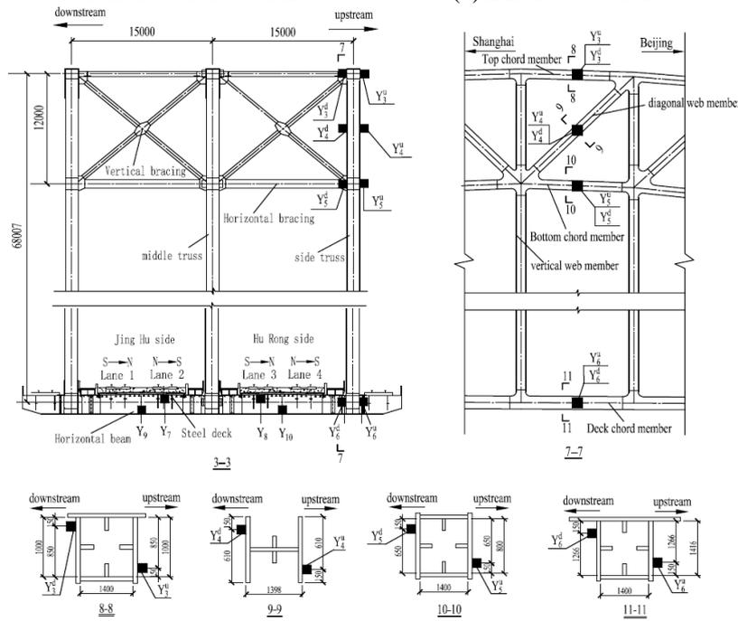
(c) 3-3 cross-section of steel truss arch
