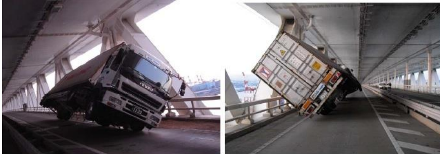
Fig. 9 Photos Rollover incident of a cargo truck on the lower deck of Yokohama-Bay Bridge during the March 11, 2011 Great East Japan Earthquake
