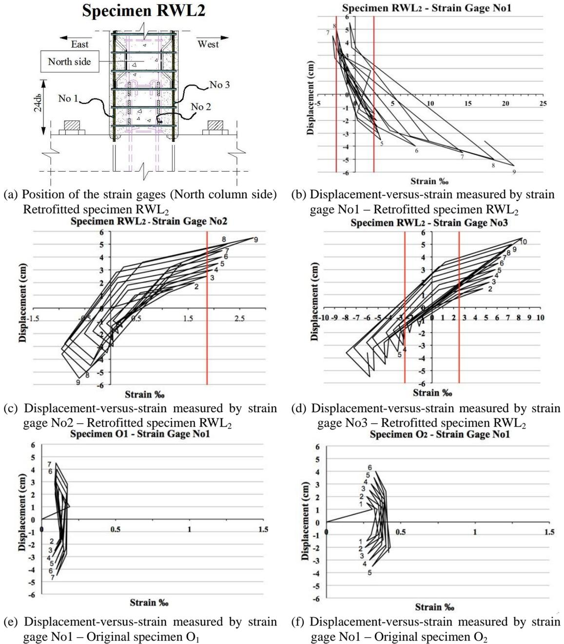
Fig. 11 Plots of displacement-versus-strain of the longitudinal reinforcement for the retrofitted specimen RWL<sub>2</sub> and the original columns O<sub>1</sub> and O<sub>2</sub>
