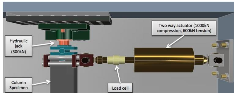
(a) Detail of the column free end - load point
