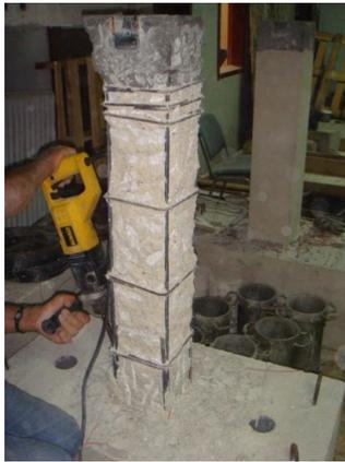
(a) the cover concrete of the original specimens is chipped away
