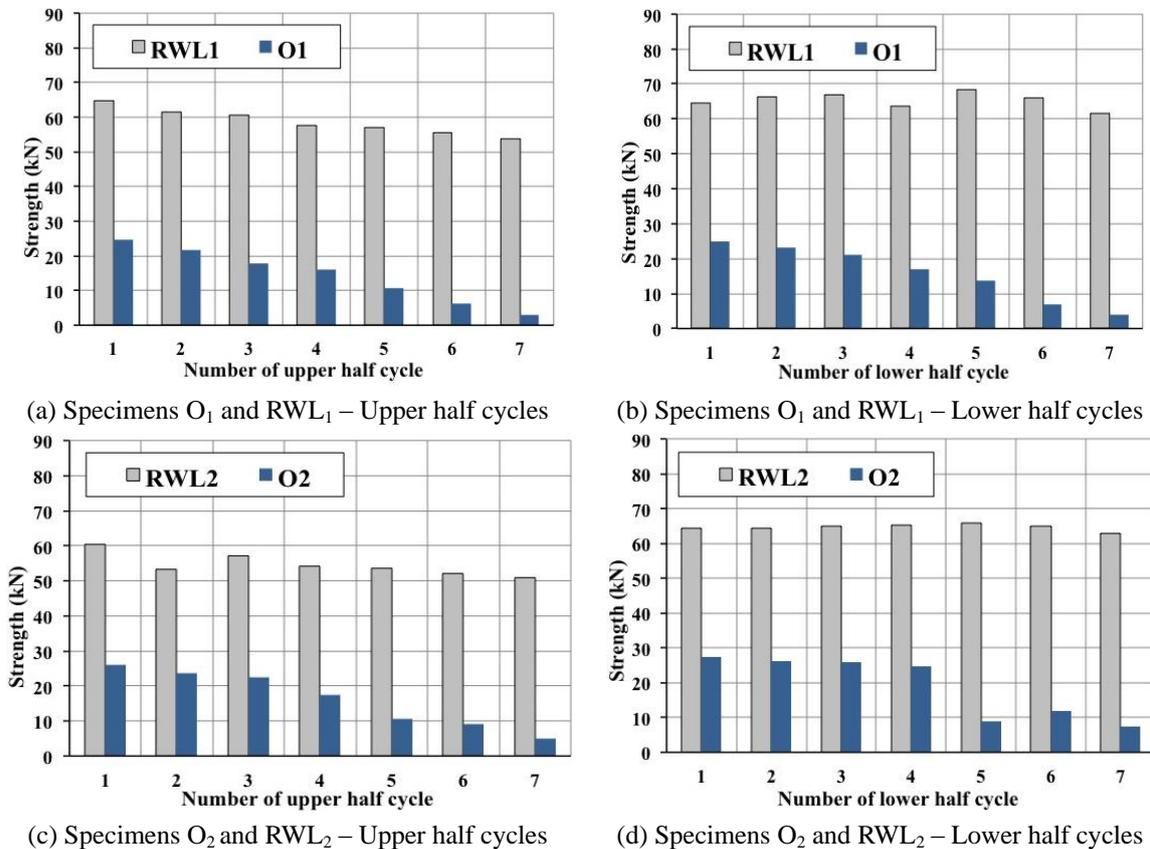
Fig. 10 Strength comparison of the original and strengthened specimens
