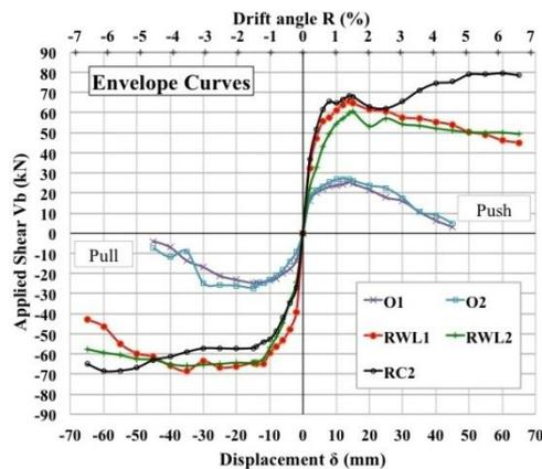
Fig. 9 Envelope curves of the original and retrofitted column sub-assemblages
