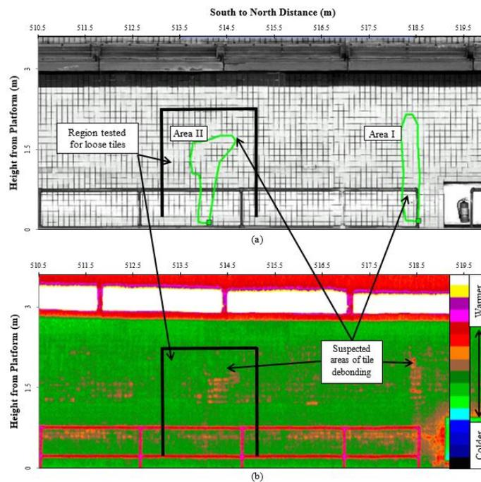
Fig. 8 SPACETEC (a) visual and (b) thermal images indicating possible tile debonding
