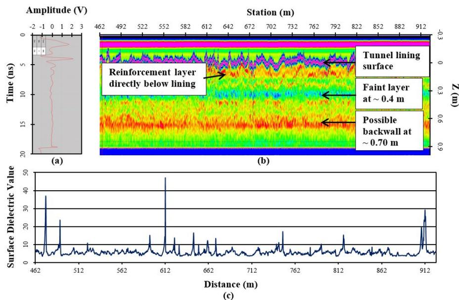
Fig. 4 GPR Data for Eisenhower Memorial Tunnel: (a) A-scan, (b) B-scan, and (c) surface dielectric
