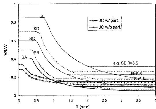
Fig. 5 Lateral load coefficient of the UBC 97 and the corresponding values of the JC (For each soil type a lower limit is set depending on  $R$ )
