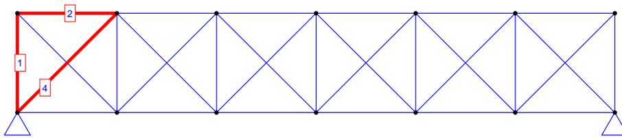
Fig. 8 Damage-suspected elements predicted for the 31-bar planar truss for damage scenario 1
