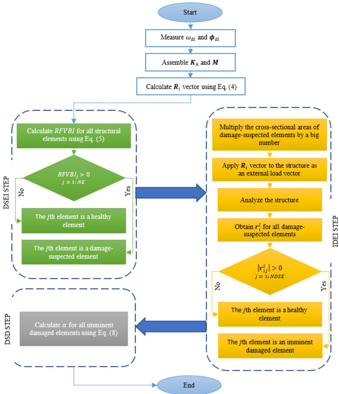
Fig. 1 Flowchart of the proposed damage detection method
