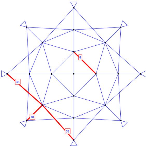
Fig. 14 Damage-suspected elements predicted for the 52-bar space truss for damage scenario 1
