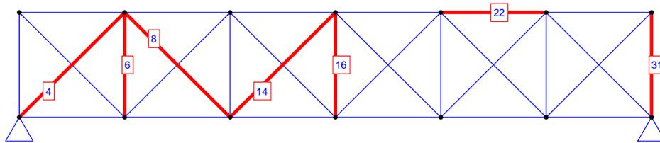
Fig. 10 Damage-suspected elements predicted for the 31-bar planar truss for damage scenario 2
