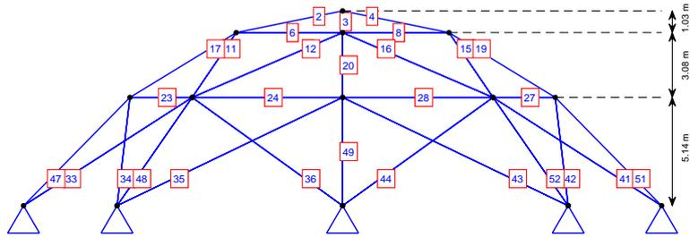
Fig. 13 Side view of the 52-bar space truss
