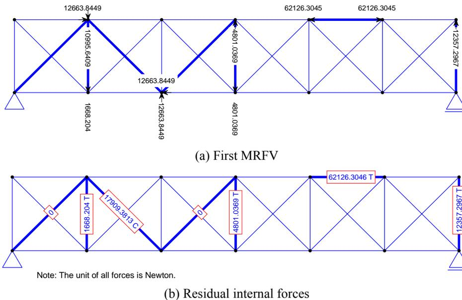
Fig. 11 First MRFV and residual internal forces for the 31-bar planar truss for damage scenario 2
