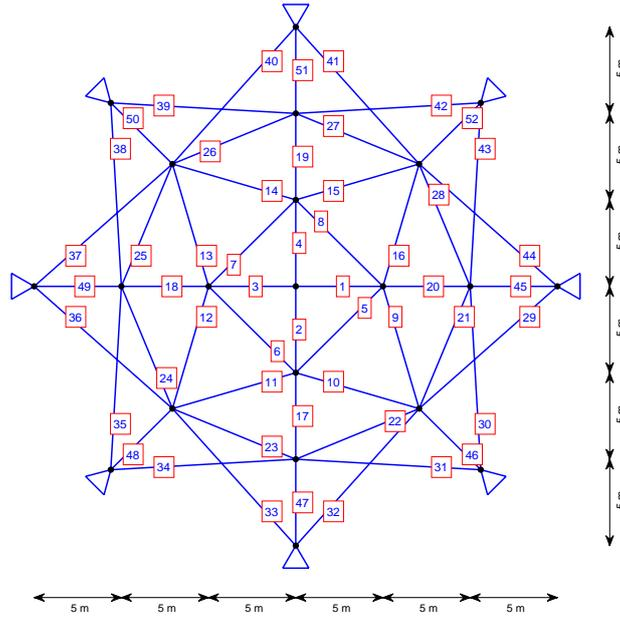
Fig. 12 Top view of the 52-bar space truss
