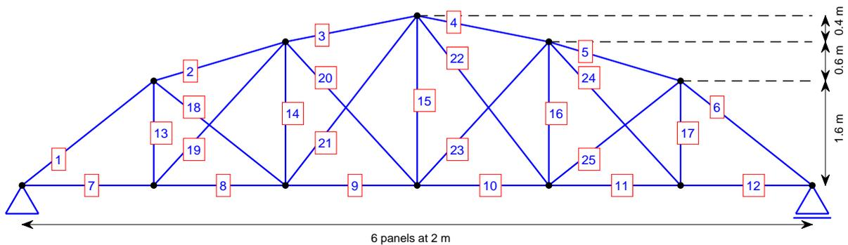
Fig. 2 The 25-bar planar truss structure
