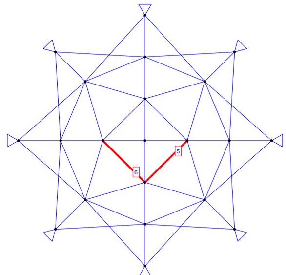
Fig. 15 Damage-suspected elements predicted for the 52-bar space truss for damage scenario 2
