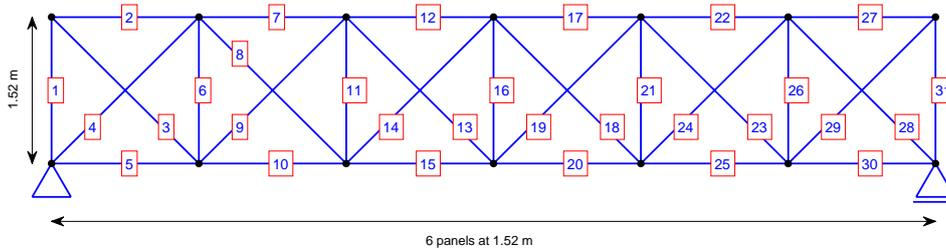
Fig. 7 The 31-bar planar truss structure
