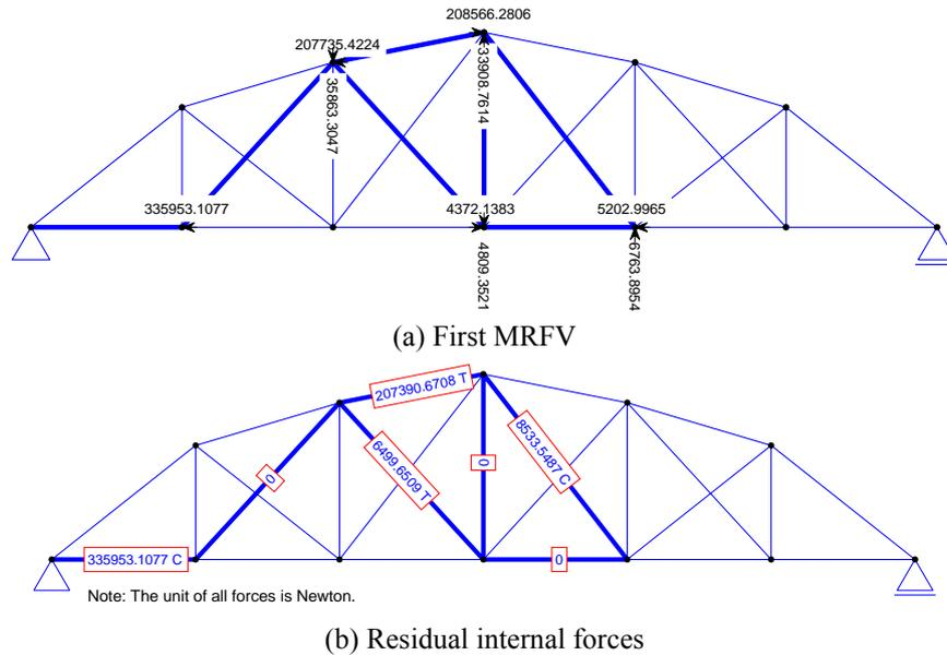
Fig. 6 First MRFV and residual internal forces for the 25-bar planar truss for damage scenario 2
