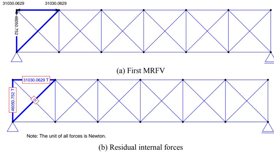
Fig. 9 First MRFV and residual internal forces for the 31-bar planar truss for damage scenario 1
