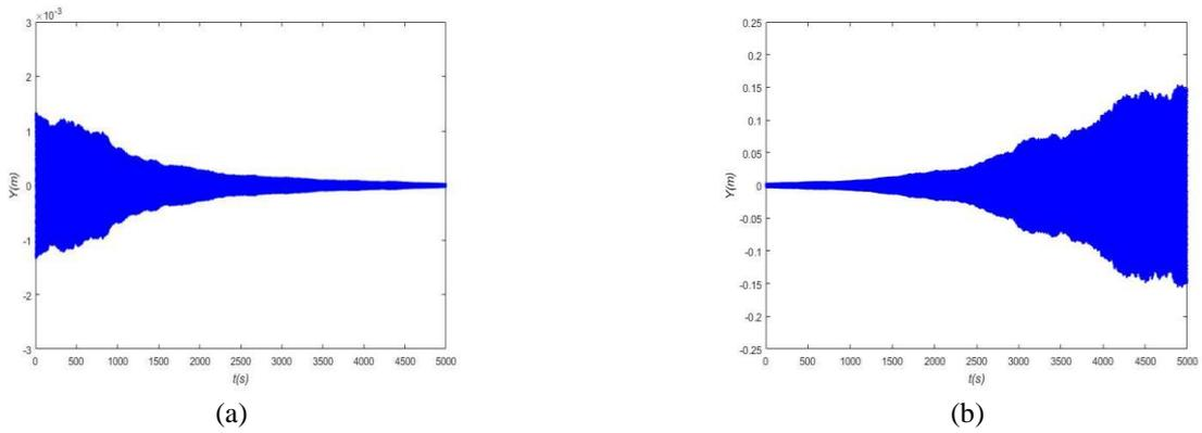
Fig. 5 Vertical displacement with different wind speeds: (a)  $U=1.6\text{m/s}$ ; (b)  $U=1.9\text{m/s}$
