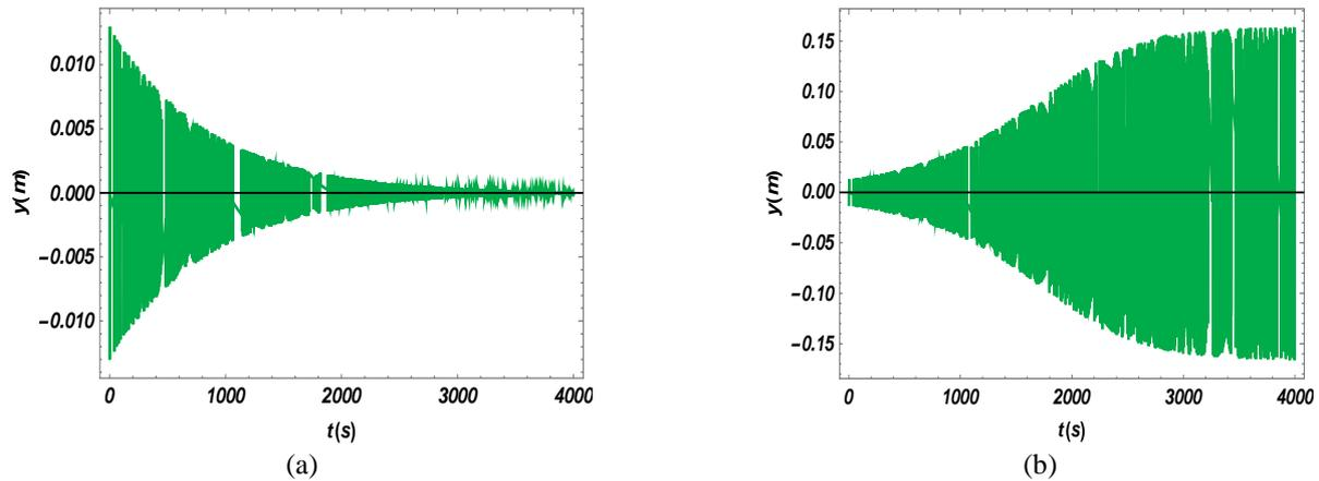
Fig. 2 Vertical displacement with different wind velocities: (a)  $U=1.6\text{m/s}$ ; (b)  $U=1.9\text{m/s}$
