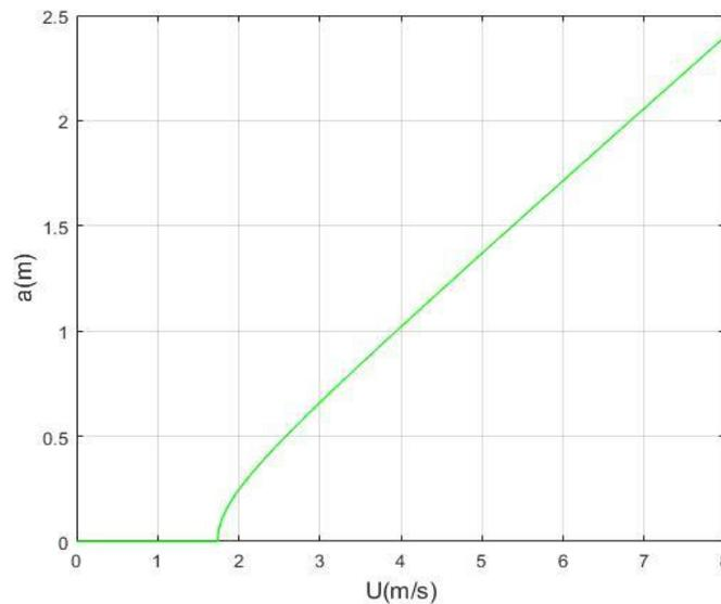
Fig. 3 The amplitude of the iced conductor with different wind velocity
