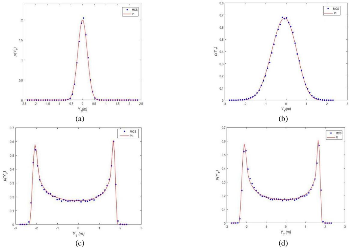
Fig. 6 Probability density of displacement at different time: (a)30s,(b)60s,(c)90s, (d)120s
