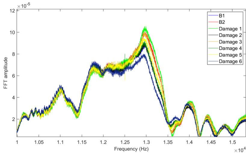
Fig. 13 The spectrums calculated by the FFT when the PZTs with 0.25” diameter were used at different artificial damage or wear levels. The excitation signal was a sweep sine wave between 100 kHz and 145 kHz
