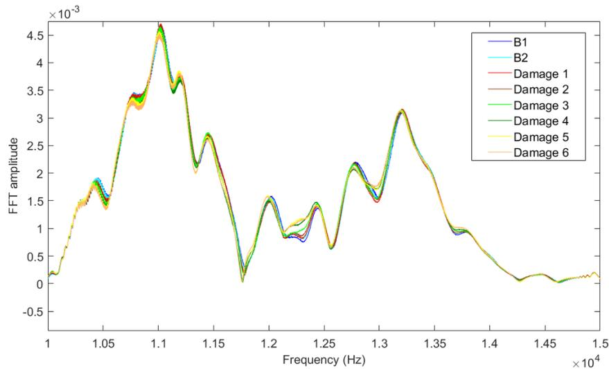
Fig. 9 The spectrums calculated by the FFT when the PZTs with 0.75" diameter were used at different artificial damage or wear levels. The excitation signal was a sweep sine wave between 100 kHz and 145 kHz
