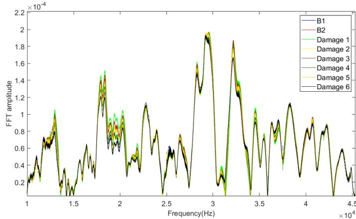
Fig. 11 The spectrums calculated by the FFT when the PZTs with 0.25” diameter were used at different artificial damage or wear levels (20 kHz and 420 kHz excitation)
