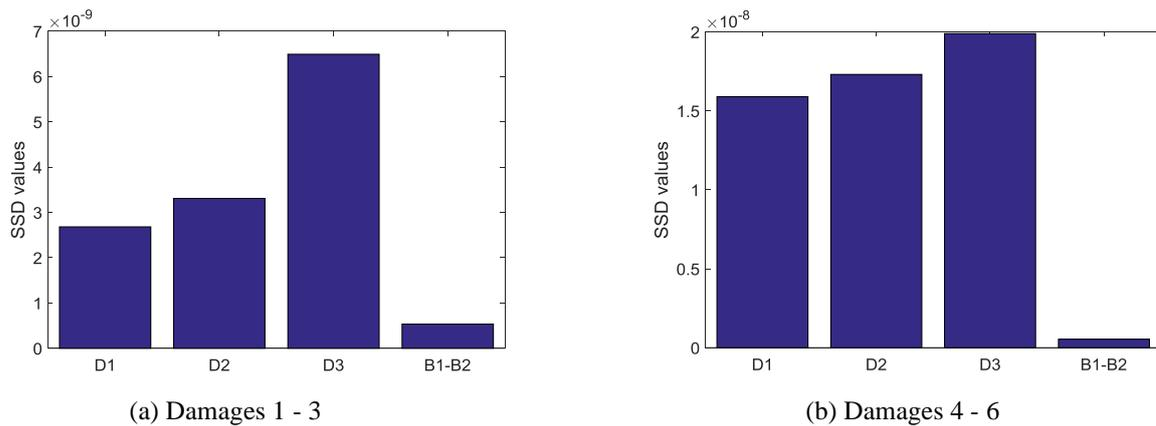
Fig. 14 SSD values for damage detection when 0.25 diameter PZTs were used. The excitation signal was sweep sine wave between 100 kHz and 145 kHz. See the Table 1 for the artificially created damage or wear information
