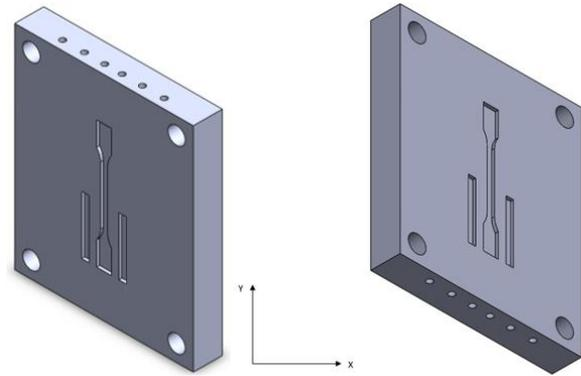
Fig. 1 3D Printed Mold
