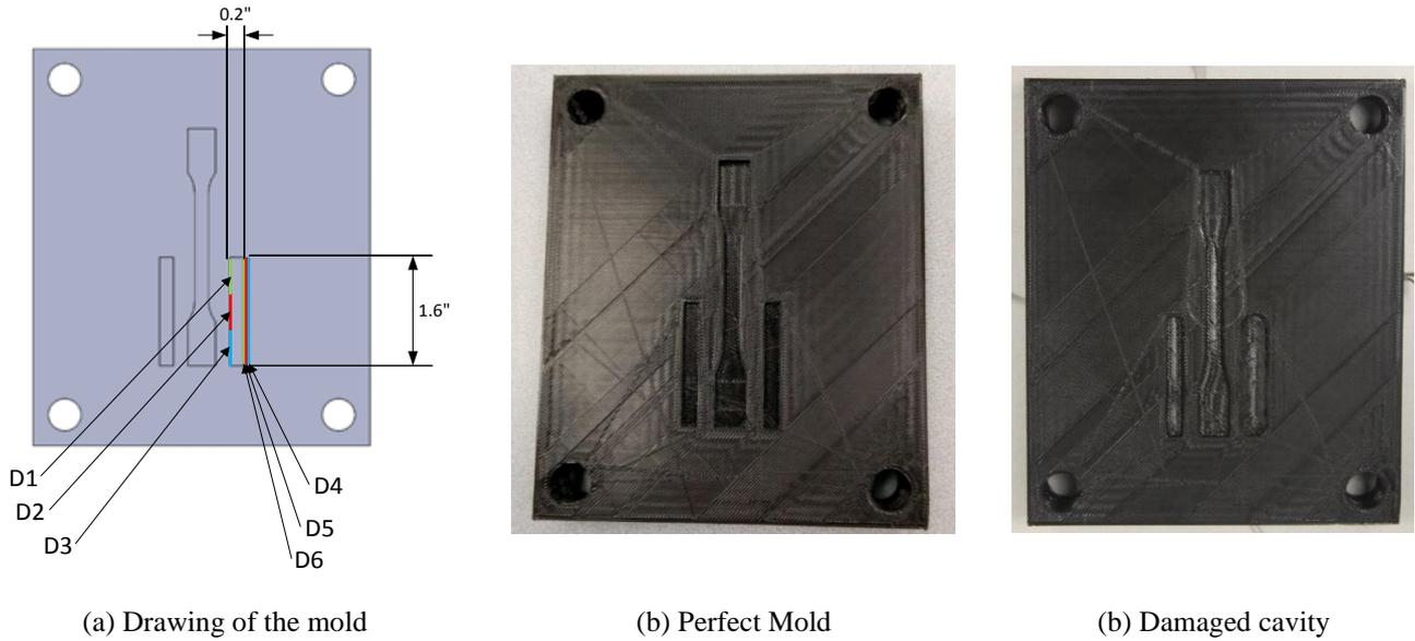
Fig. 8 Created damage shown in three colors
