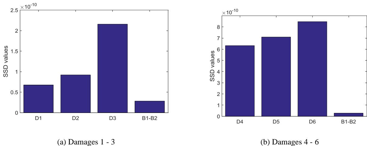
Fig. 10 SSD values for damage detection when 0.75 diameter PZTs were used. The excitation signal was a sweep sine wave between 100 kHz and 145 kHz. See the Table 1 for the artificially created damage or wear information
