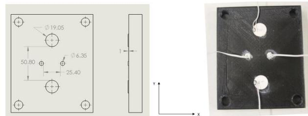
Fig. 2 Drawing (left) and actual part with PZTs (right) of attached PZTs on the back of the 3D printed mold (The unit dimension is millimeter)
