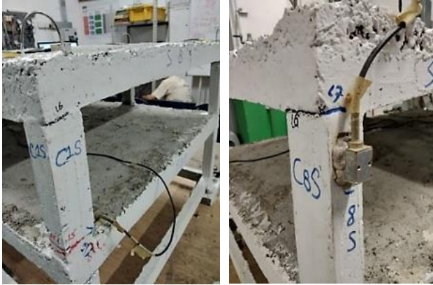
Fig. 20 Flexural horizontal cracks at roof beam column joint
