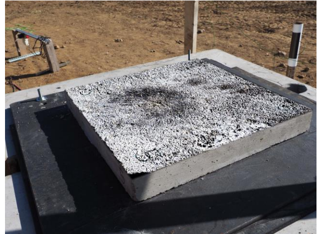
Fig. 8 Blackened pattern from the explosion of an incorrectly placed charge (adjusted contrast)
