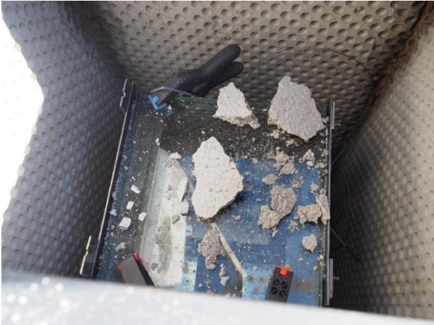
Fig. 4 Laser sensor inside the column base protected with Plexiglass
