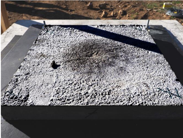
Fig. 6 Blackened pattern from the explosion (adjusted contrast)
