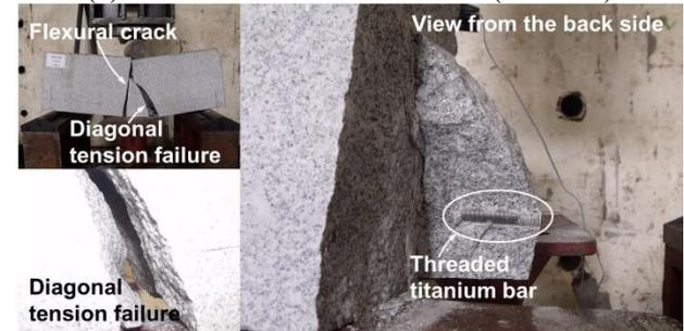
(b) Flexural and diagonal tension failure (SP16-50)
