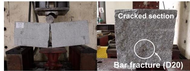
(a) Flexural crack and bar fracture (SP20-90)
