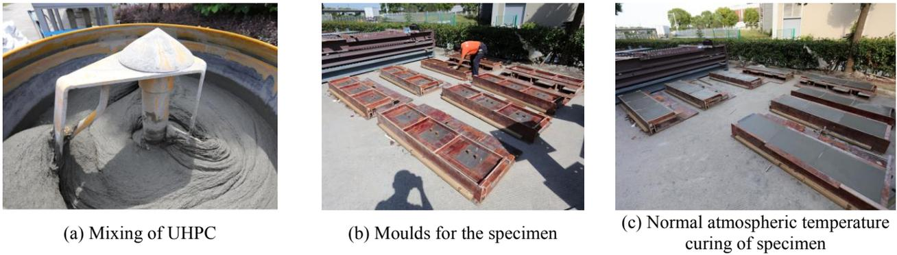
Fig. 3 Manufacture of push-out test specimens
