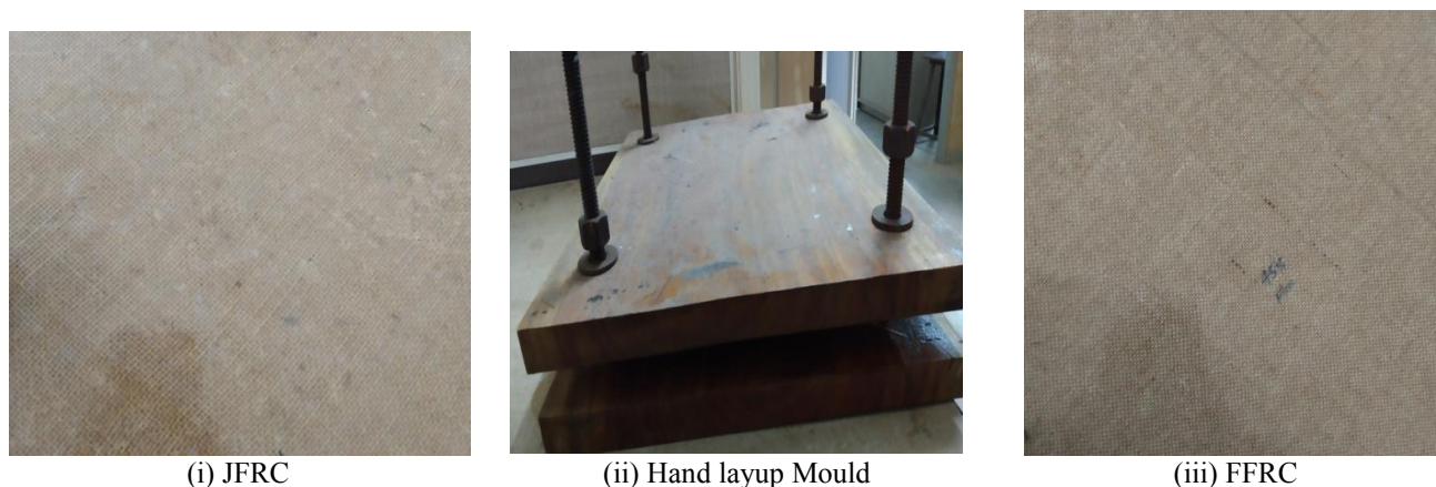
Fig. 2 (i) Jute fibre reinforced composite plate, (ii) Mould box, (iii) Flax fibre reinforced composite plate
