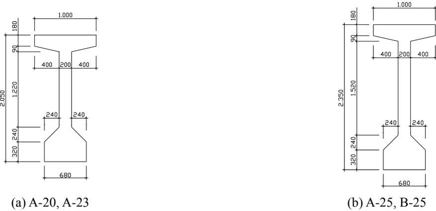
Fig. 6 Details of girder sections (units: mm)
