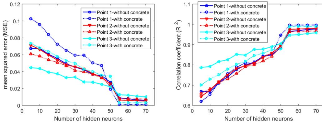
Fig. 4 The Performance of ANN structures with different number of hidden neurons. Each result in the graph is the best result for its ANN structure determined over 20 Trials. (A) Changing of MSE with respect to number of hidden neurons (B) Changing of coefficient with respect to number of hidden neurons
