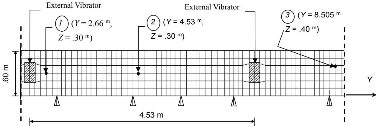
Fig. 1 Measurement surface of finite element mesh of Column mold (Y-Z Plane, X = .30 m)
