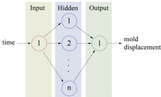
Fig. 3 Proposed structure of ANN Model. Number of Neurons in Hidden Layer Is  $N=5:5:70$
