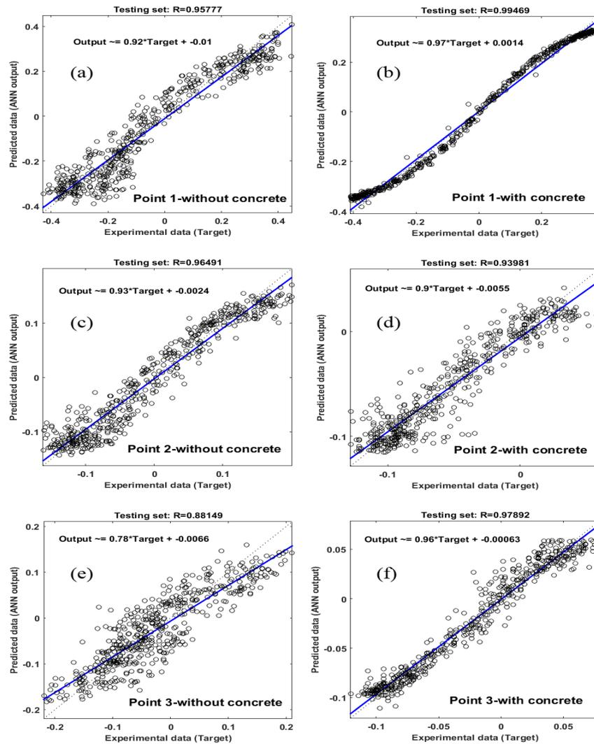
Fig. 5 Comparison of experimental and predicted mold displacement data in the testing stage
