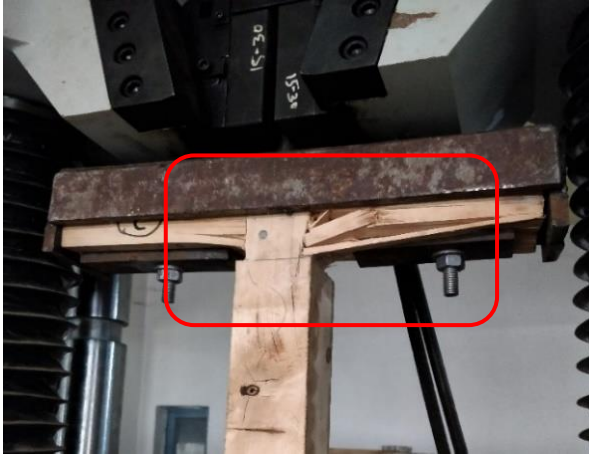
Fig. 18 Heavy Cross Grain Splitting in DH*2
