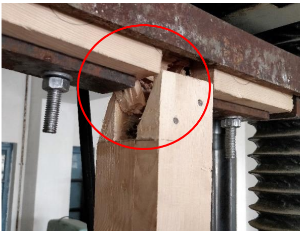
Fig. 19 Horizontal Member Tear Out in BT*4
