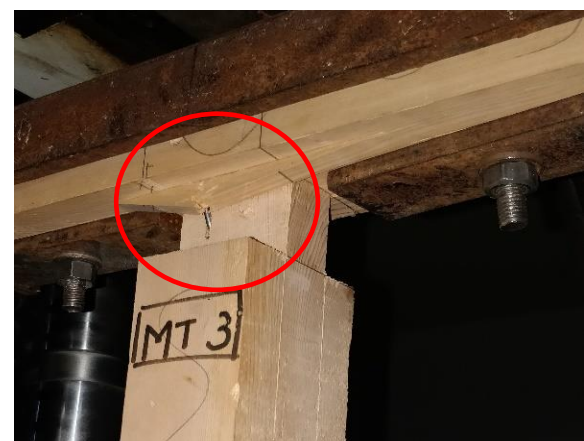
Fig. 23 Mortise Splitting in MT-3
