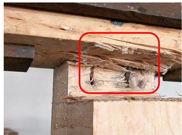
Fig. 22 Shear Bearing Failure in CH*2
