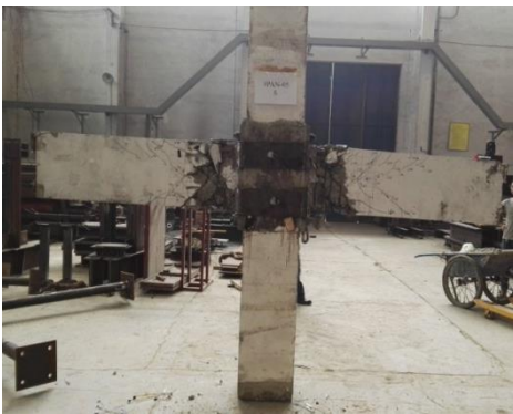
(a) #PAN-05 ultimate failure diagram
