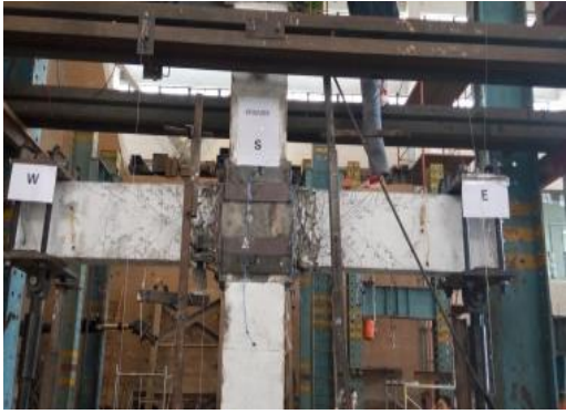
(b) #PAN-08 ultimate failure diagram
