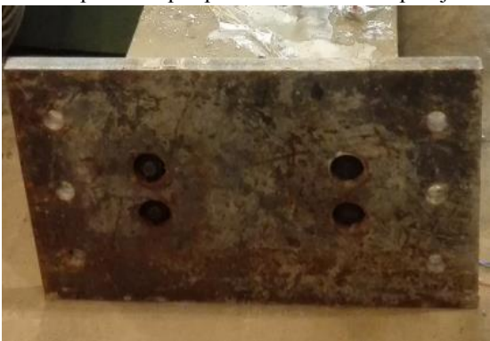
(e) The prestressed reinforcements are anchored inside the end plate by nut
