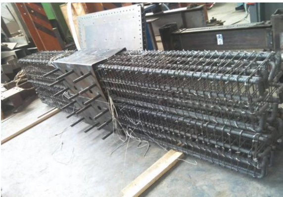
(c) The steel plate hoop replace common stirrup in joint zone
