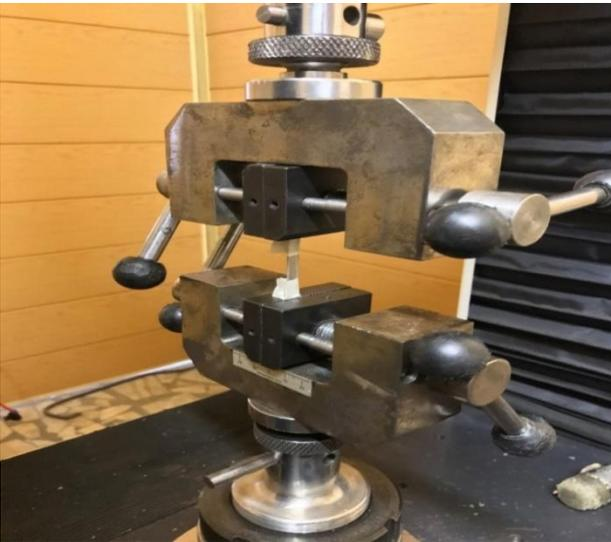
Fig. 17 Standard tensile test
