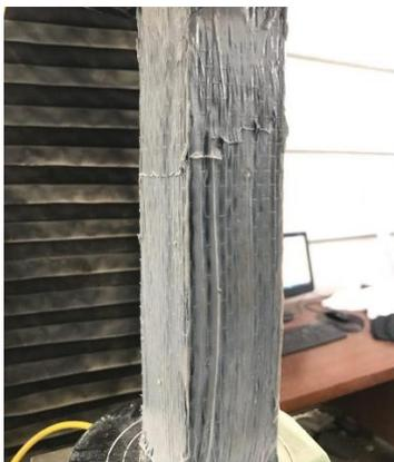
Fig. 11 Small cracks in groups 7 and 8, b. Diagonal cracks in group 8
