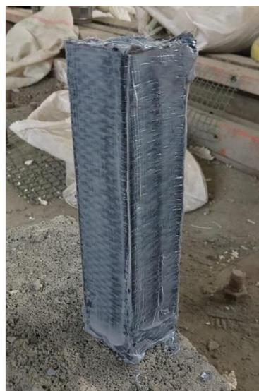
Fig. 2 Rectangular timber columns confined with FRP sheets
