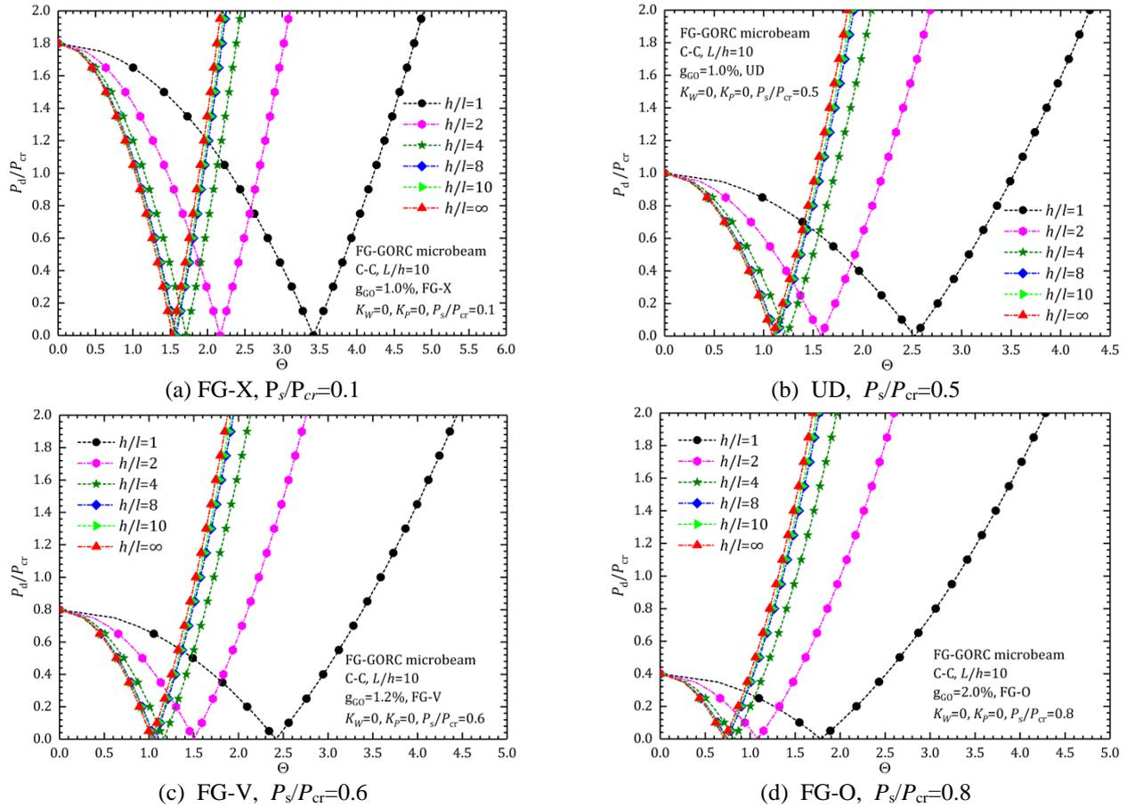
Fig. 2 Effects of the microbeam size on the unstable region of the FG-GORC microbeam
