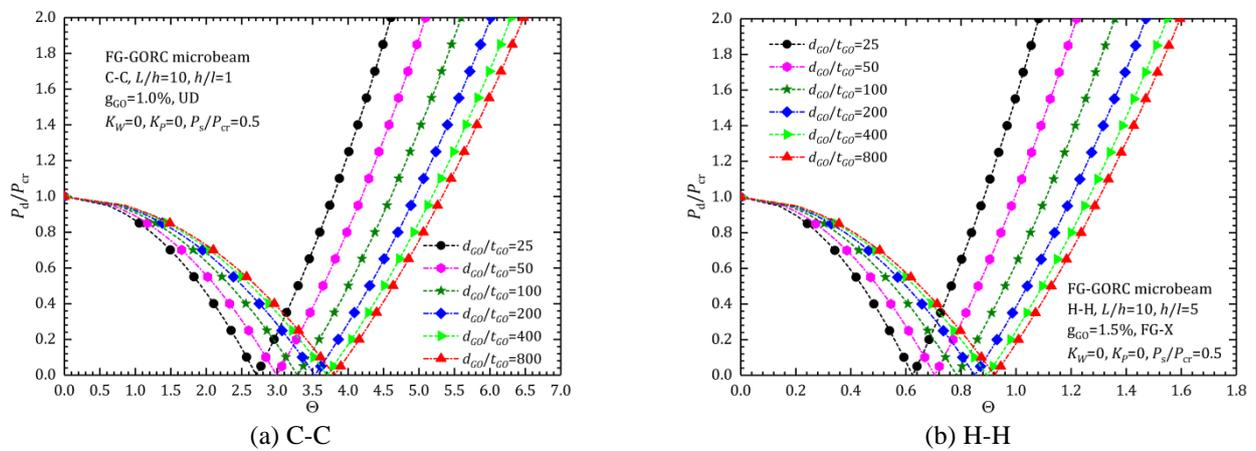
Fig. 6 Effects of the particle diameter-to-thickness ratio ( $d_{GO}/t_{GO}$ ) on the principal unstable region of the FG-GORC microbeams
