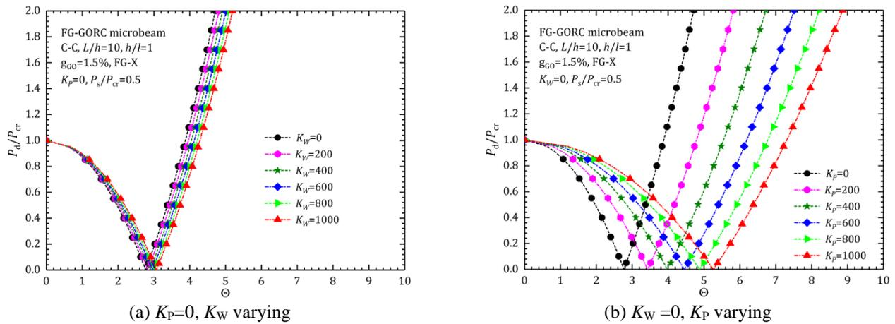
Fig. 7 Effects of the elastic substrate on dynamic stability of FG-GORC microbeams
