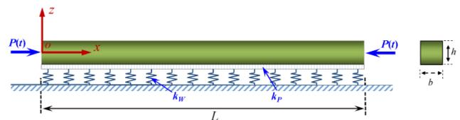
Fig. 1 Schematic of a FG-GORC beam rests on a Winkler–Pasternak elastic substrate
