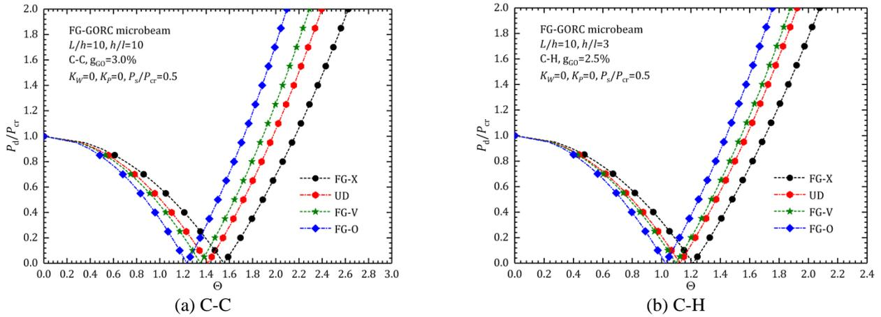
Fig. 5 Effects of the GO distribution on the dynamic stability of FG-GORC microbeams
