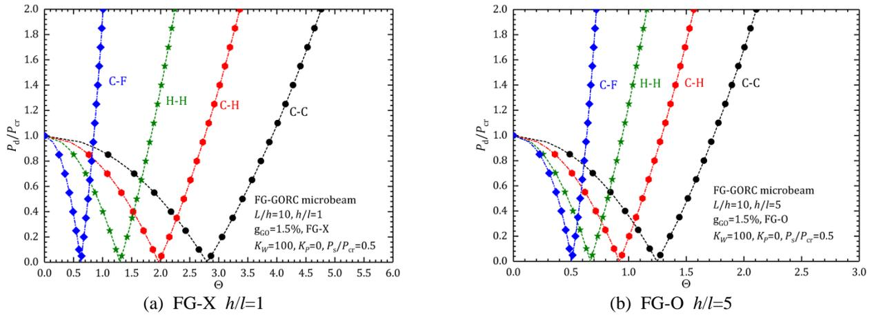
Fig. 3 Effects of the boundary conditions on the unstable region of the FG-GORC microbeam
