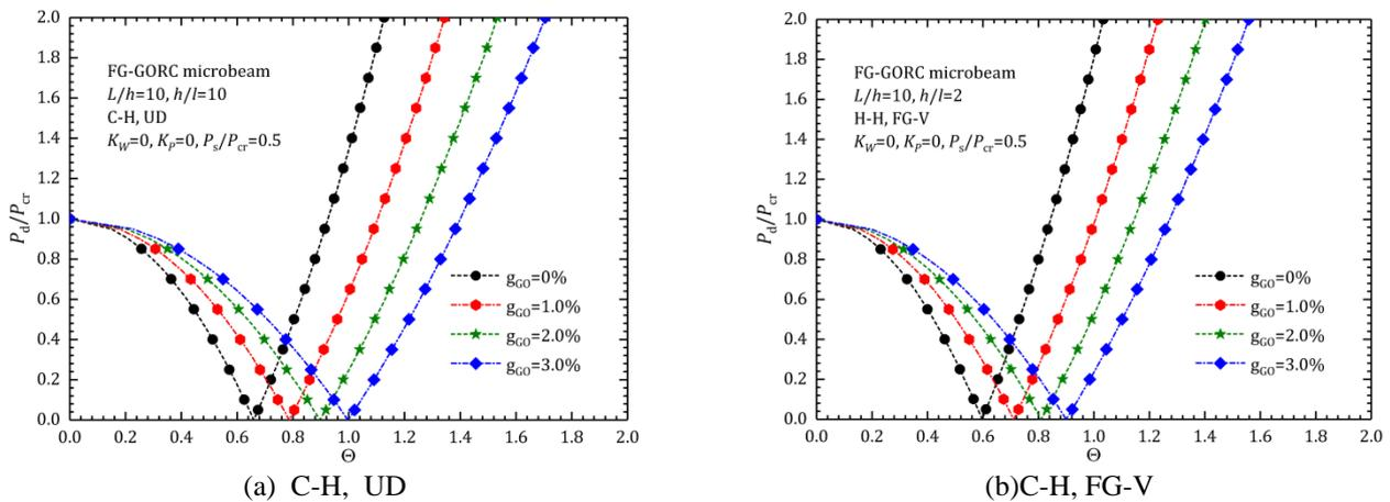
Fig. 4 Effects of the GO weight fraction on the dynamic stability of FG-GORC microbeams
