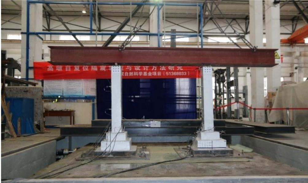
Fig. 8 Arrangement of the shaking table test
