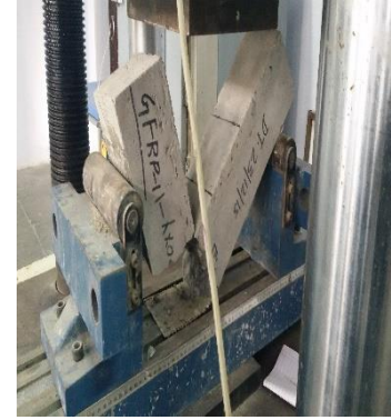
Fig. 6 FRP wrapped prisms
