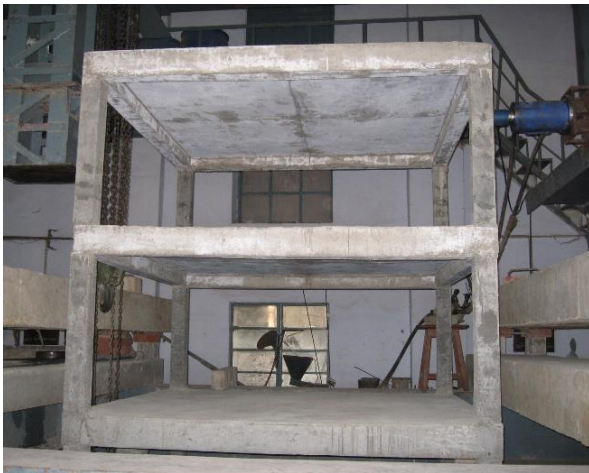
Fig. 2 Actual RC Bare Frame used in the study
