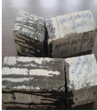
Fig. 5 Failure of Epoxy jointed Prisms
