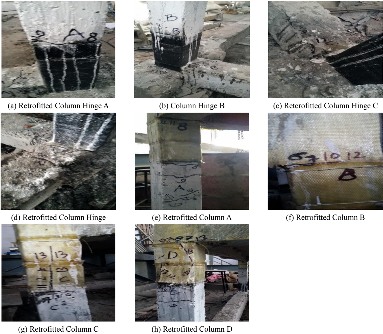
Fig. 20 Damage in Column-Beam and Column-Foundation after loading in Retrofitted Brick infilled frame
