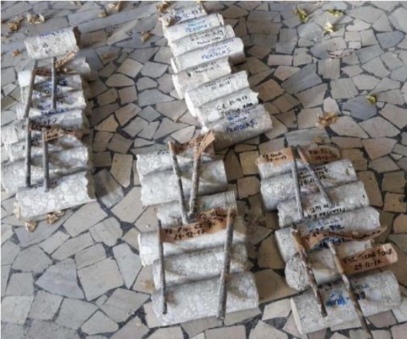
Fig. 3 Concrete cores and steel bars extracted and tested in the case study
