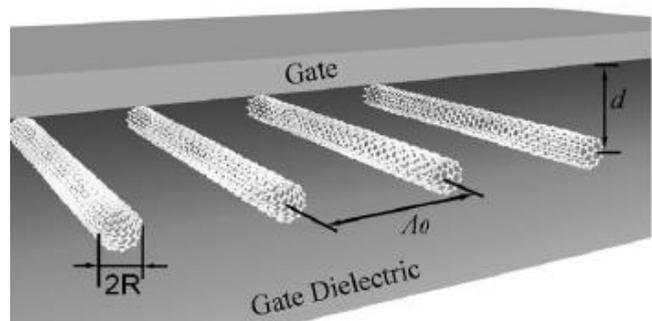
Fig. 1 Model of the thin-film transistors ( $R$ : nanotube radius,  $d$ : distance between each tube,  $\lambda_0$ : dielectric thickness) (Cao *et al.* 2007)
