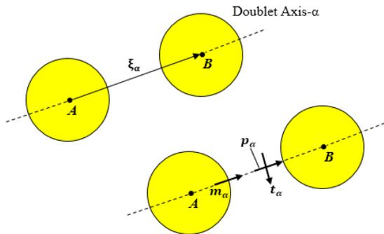
Fig. 2 Micro stresses in a doublet geometry (Ferrari *et al.* 1997)
