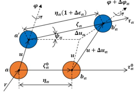
Fig. 3 Deformation of the doublet nodes (Ferrari *et al.* 1997)
