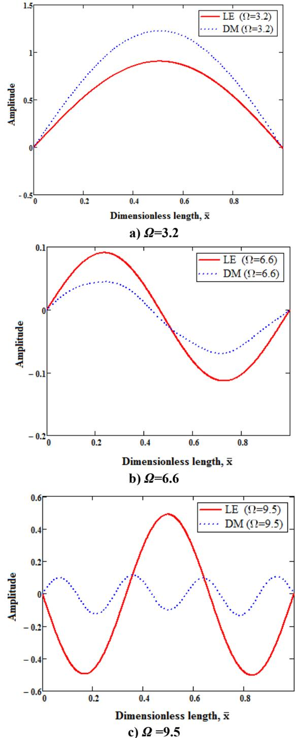
Fig. 17 Relative mode shapes of DNRS under linear axial load at C-C boundary condition ( $L=1$  nm,  $K=0.5$ )
