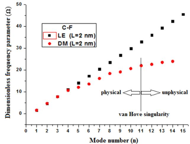
Fig. 8 Variation of dimensionless frequency parameter with mode number for C-F DNRS ( $K=0$ )
