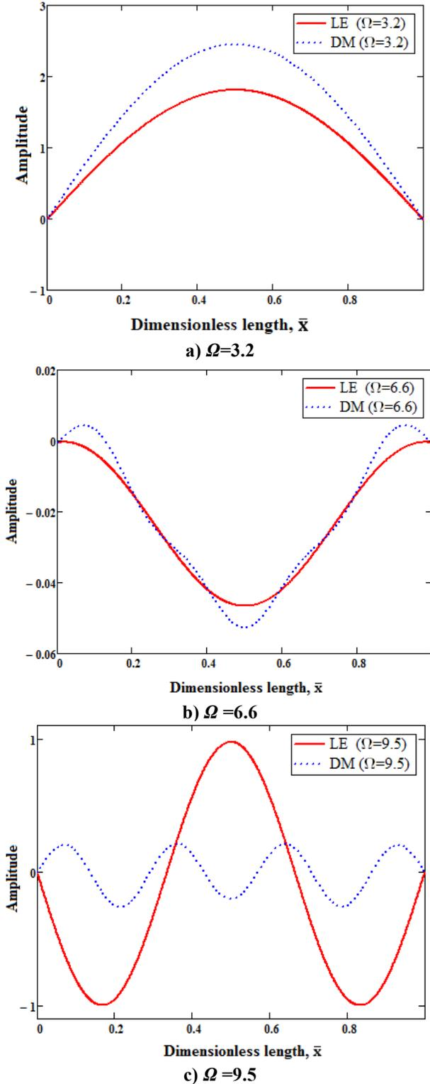
Fig. 16 Relative mode shapes of DNRS under uniform axial load at C-C boundary condition ( $L=1$  nm,  $K=0.5$ )
