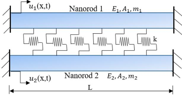
Fig. 5a A DNRS for C-C boundary conditions
