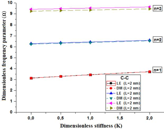
Fig. 10 Variation of dimensionless frequency parameter with dimensionless stiffness for the first three modes for C-C DNRS
