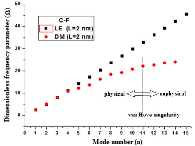
Fig. 9 Variation of dimensionless frequency parameter with mode number for C-F DNRS ( $K=2$ )
