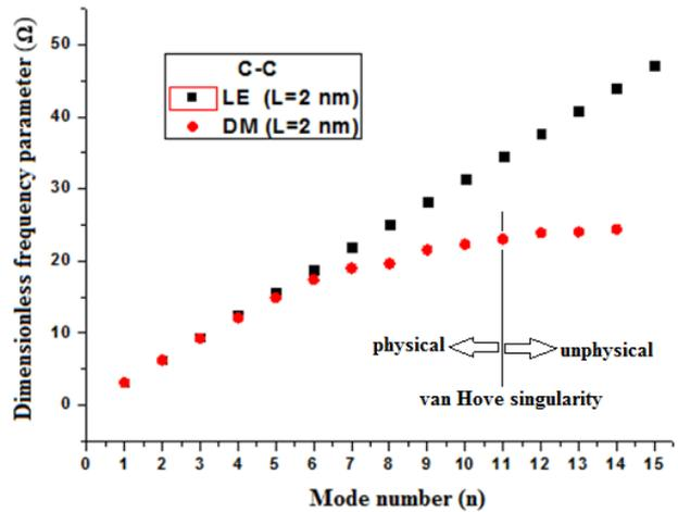
Fig. 6 Variation of dimensionless frequency parameter with mode number for C-C DNRS ( $K=0$ )
