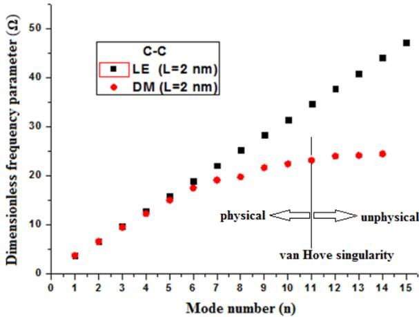
Fig. 7 Variation of dimensionless frequency parameter with mode number for C-C DNRS ( $K=2$ )
