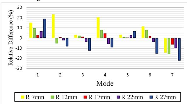
Fig. 10 Relative difference of eigenfrequencies of five FE models
