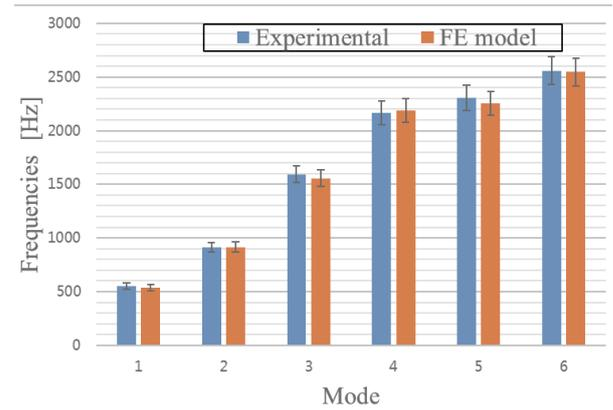
Fig. 7 Platform only: frequency-comparison for correlated mode shapes
