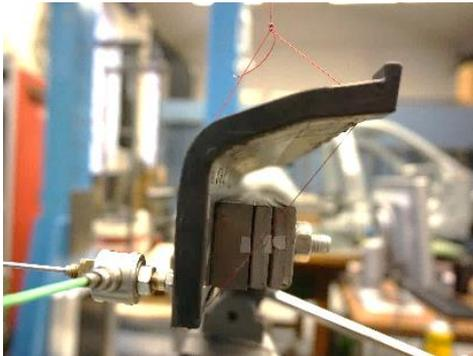
(a) Side-view, connection force transmitter to damper
