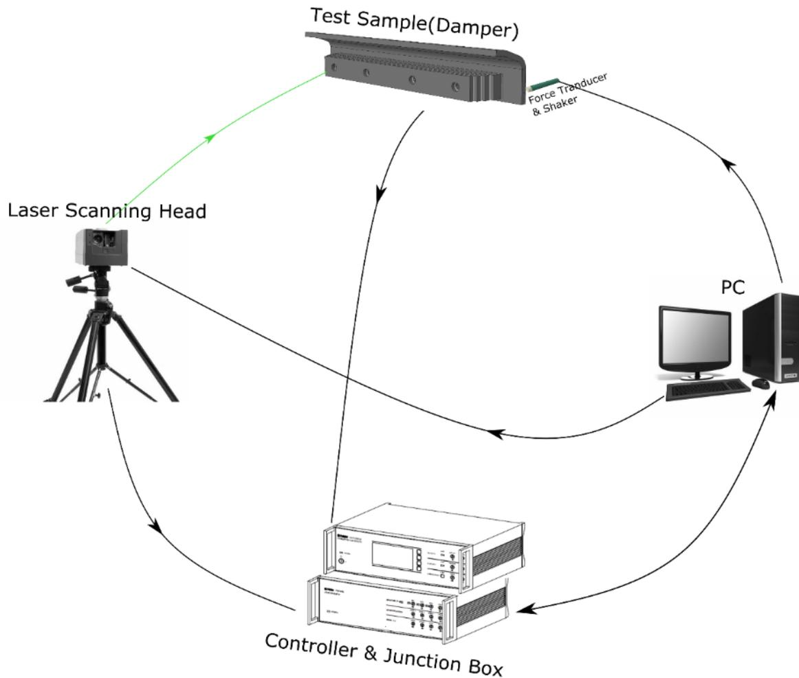
Fig. 4 Experimental equipment and schematic setup for the rail damper modal analysis
