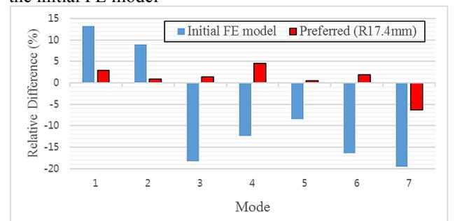
Fig. 12 Relative difference of eigenfrequencies the preferred and the initial FE model
