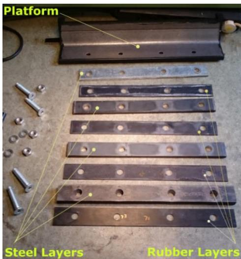
Fig. 2 Unassembled damper to check friction between the layer
