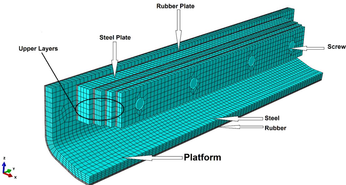
Fig. 1 FE model of rail damper with components including platform, upper layers (steel layers, rubber layers) and screws
