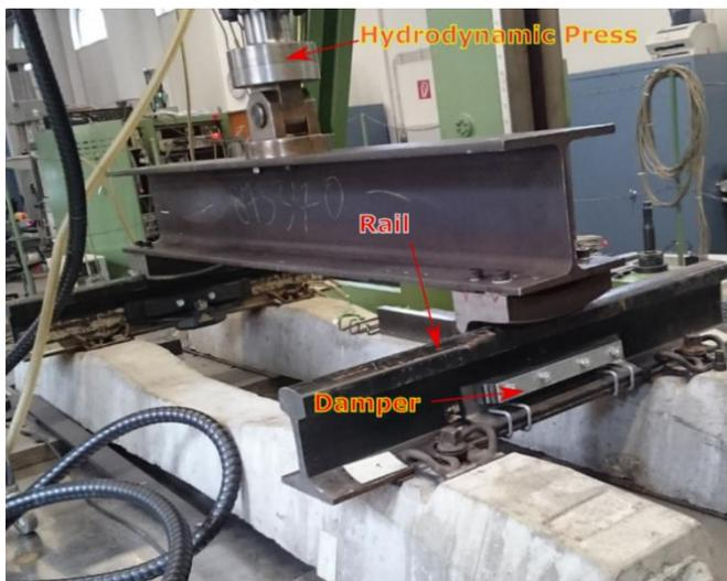
Fig. 3 Cycle test on one-meter rail and damper
