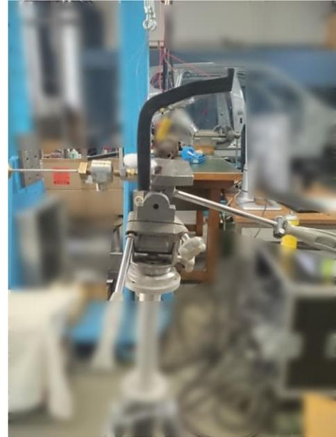
Fig. 6 Modal test, only platform of damper
