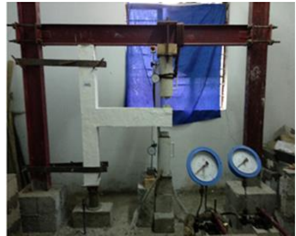
Fig. 3 Testing of beam-column connection (a) Test set-up (b) Actual testing arrangement
