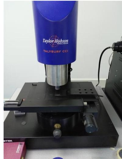
(a) White-light optical interferometer system
