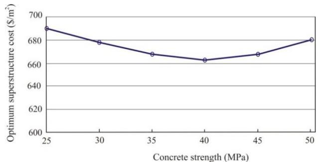
Fig. 13 Effect of concrete strength on optimum superstructure cost
