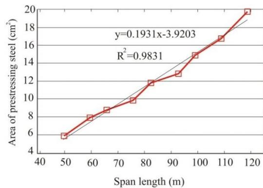
Fig. 14 Relation between prestressing tendons cross-sectional area and span length
