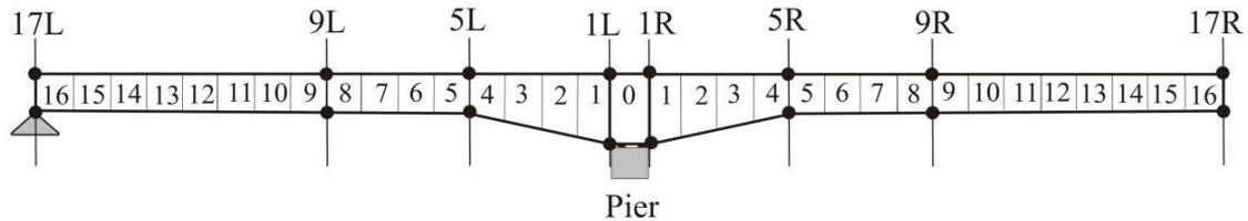
Fig. 6 Installation sequence of segments and critical sections
