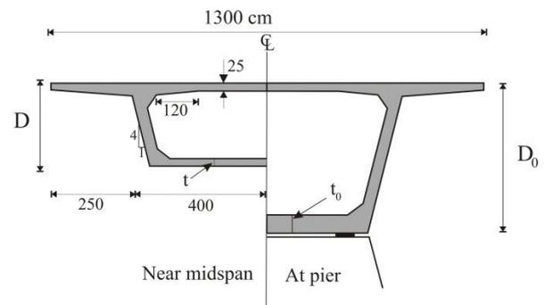
Fig. 2 Typical cross-section of deck bridge
