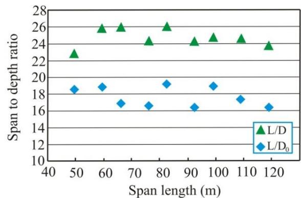
Fig. 11 Span/depth ratio at piers and mid-span for different span length
