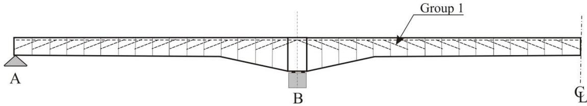
Fig. 3 Group1: Cantilever tendon layout
