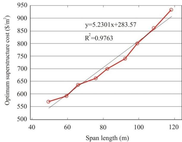
Fig. 12 Relation between optimum cost and span length
