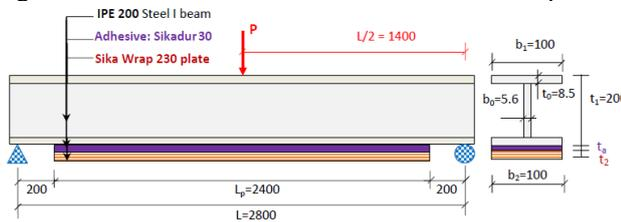
Fig. 4c Steel beam reinforced with four layers of Sika Wrap
