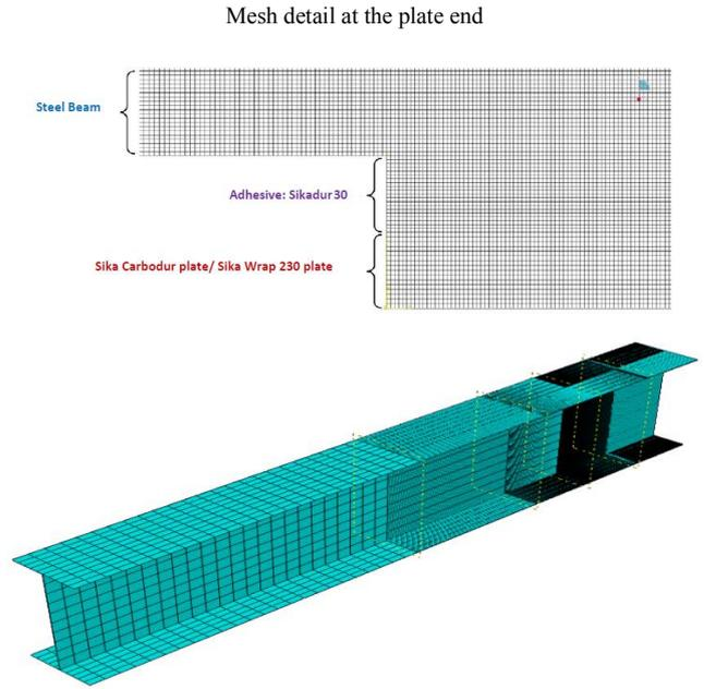
Fig. 3 FE mesh of Mesh of an “IPE” steel beam
