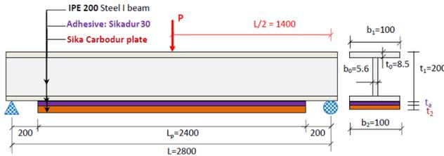
Fig. 4b Steel beam reinforced with a Sika carbodur plate
