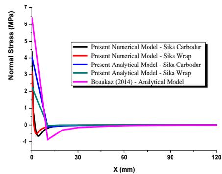
Fig. 8 Comparison of interfacial normal stress for the steel beams reinforced with composite plate
