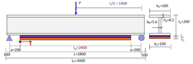
Fig. 1 steel beam strengthened with a bonded composite plate loaded with a concentrated load P at mid-span
