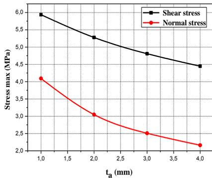
Fig. 9 Effect of adhesive layer thickness on interfacial stress at the ends of bonded sika carbodur plate
