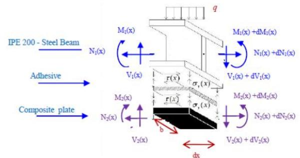
Fig. 2 Steel beam simply supported reinforced with composite plate bonded and loaded by a uniformly distributed load
