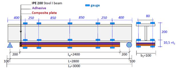
Fig. 5 Strains gages locations for the steel beams reinforced with composite plate.
