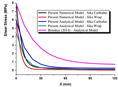
Fig. 7 Comparison of interfacial shear stress for the steel beams reinforced with composite plate
