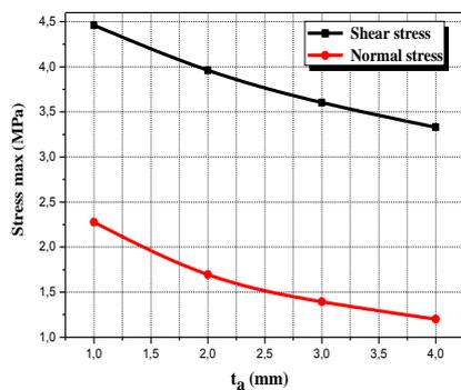
Fig. 10 Effect of adhesive layer thickness on interfacial stress at the ends of bonded sika wrap plate
