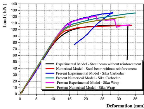
Fig. 6 Experimental and numerical comparison for the steel beams reinforced with composite plate
