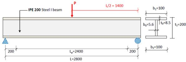
Fig. 4a Steel beam without reinforcement “Reference Beam”
