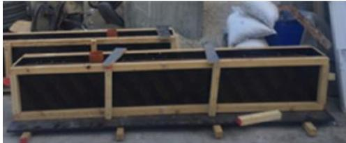
Fig. 5 Formwork of beams samples and installed vertical pipe for the experiment
