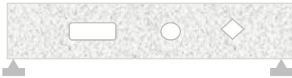
Fig. 1 RC beams with different types of openings
