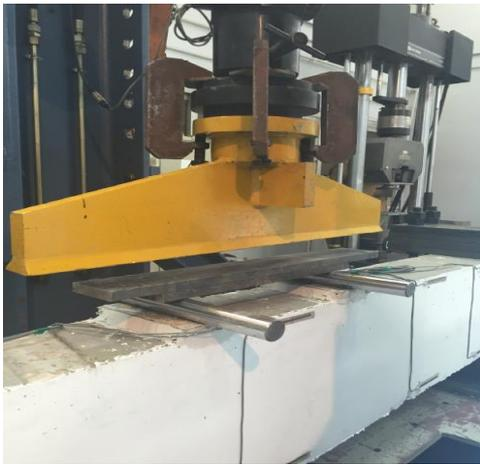
Fig. 6 The structural testing test set up for the beam
