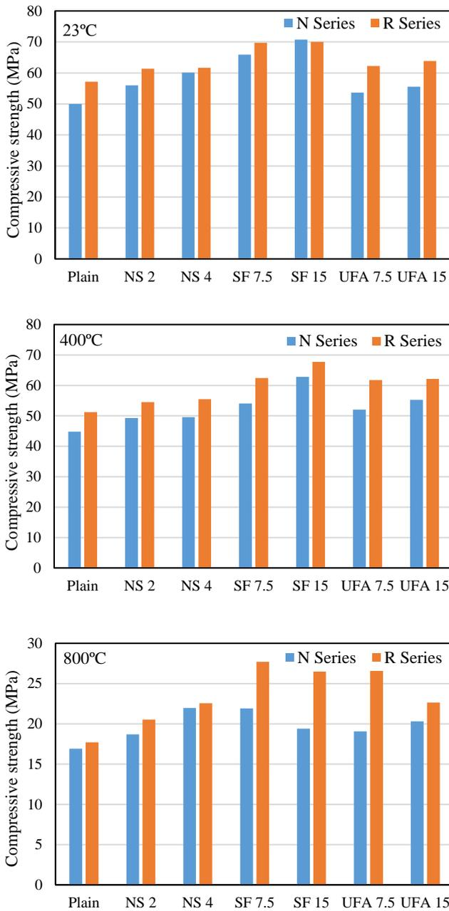
Fig. 5 Effect of different types of fine aggregate on compressive strength for each thermal group
