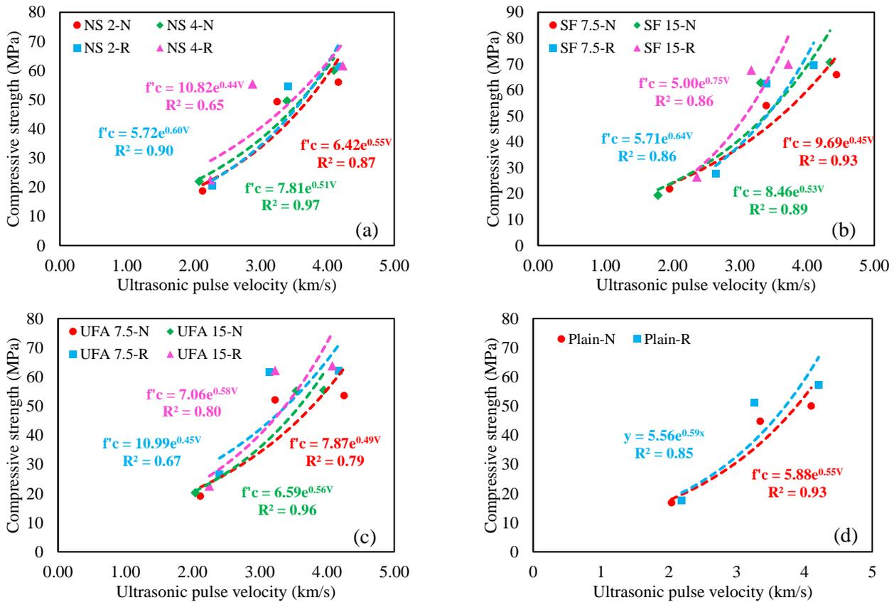
Fig. 12 Empirical relationships between compressive strength and UPV for different mixes; (a) nanosilica, (b) silica fume, (c) ultrafine fly ash, and (d) plain
