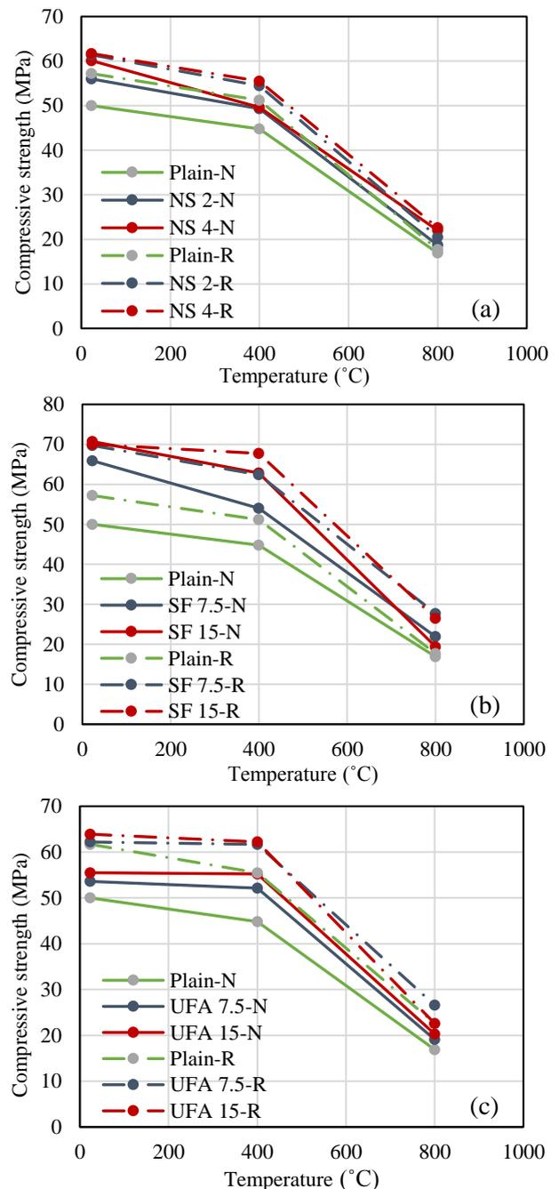
Fig. 6 Effect of different pozzolan types on compressive strength; (a) nanosilica, (b) silica fume, and (c) ultrafine fly ash
