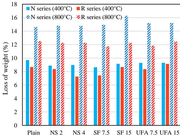
Fig. 8 Loss of weight of mixtures exposed to elevated temperatures
