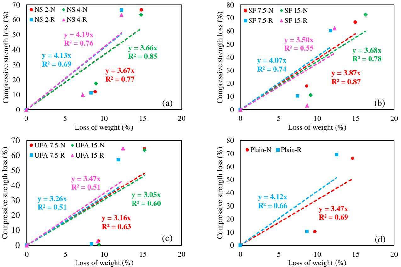
Fig. 9 Relationship between weight loss and compressive strength loss of different mixes; (a) nanosilica, (b) silica fume, (c) ultrafine fly ash, and (d) plain
