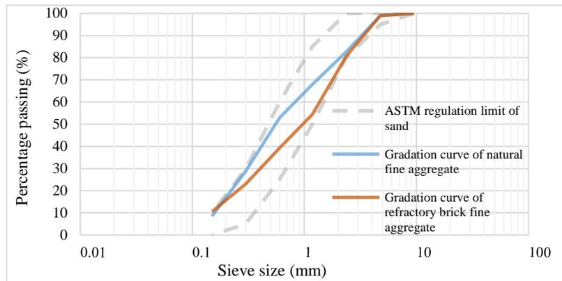
Fig. 2 Grading curves of natural and recycled refractory brick fine aggregates
