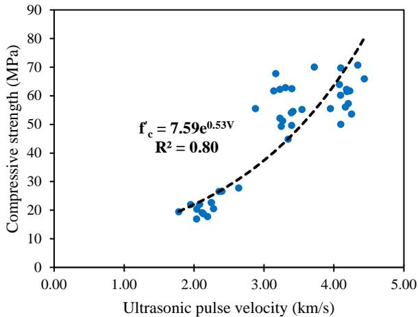
Fig. 13 General empirical relationship between compressive strength and UPV
