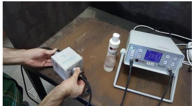
Fig. 4 Ultrasonic pulse test apparatus and attachment of transducers to surface of specimens
