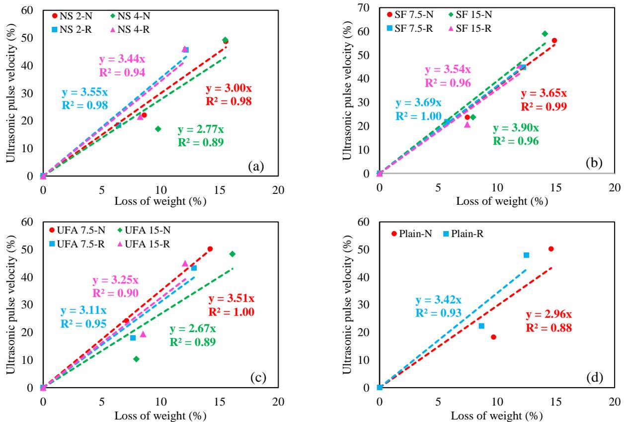
Fig. 11 Relationship between weight loss and ultrasonic pulse velocity loss of different mixes; (a) nanosilica, (b) silica fume, (c) ultrafine fly ash, and (d) plain
