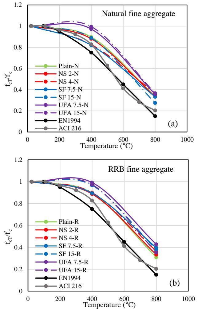
Fig. 7 Normalized compressive strength of concrete as a function of temperature; (a) mixtures containing natural fine aggregate and (b) mixtures containing RRB fine aggregate
