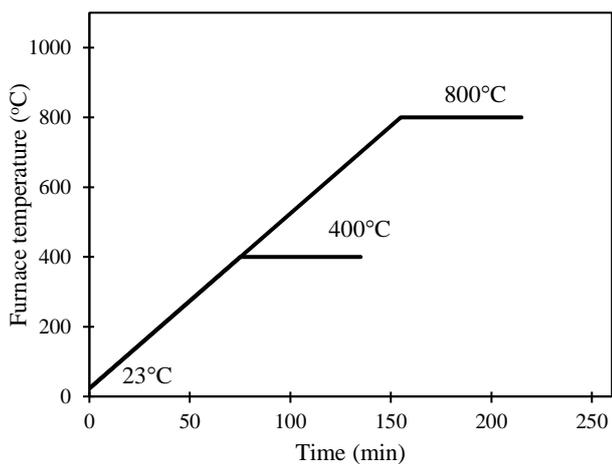
Fig. 3 Heating regimes inside electric furnace applied to concrete specimens
