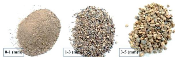
Fig. 1 Different grain sizes of refractory brick aggregate
