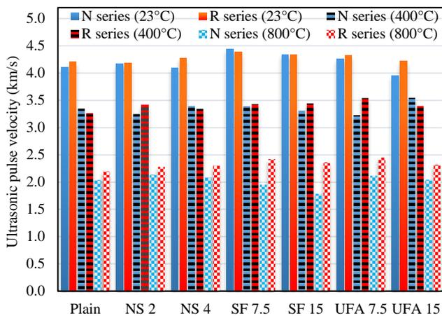
Fig. 10 Ultrasonic pulse velocity of mixes exposed to elevated temperatures
