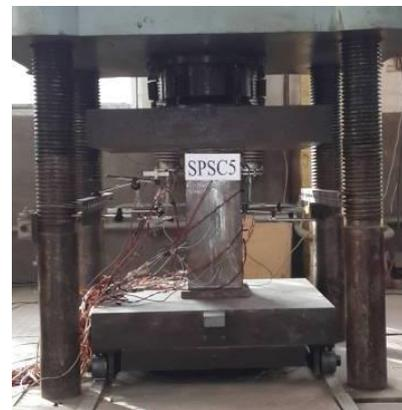
Fig. 2 Loading devices of axial compression tests
