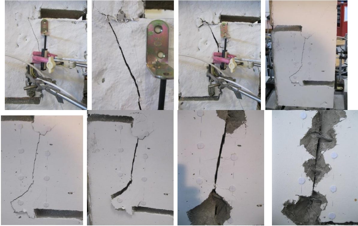
Fig. 7 Crack sequence on both sides of a specimen with fiber and with steel reinforcement crossing the shear plane (Specimen SHCC-S)
