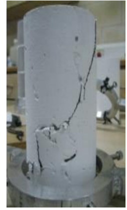
(c) failure cracks for SHCC
