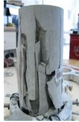
(b) failure cracks for HVFA
