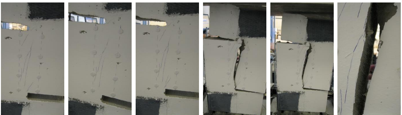
Fig. 6 Crack sequence on both sides of a specimen with fiber but without steel reinforcement crossing the shear plane (Specimen SHCC)
