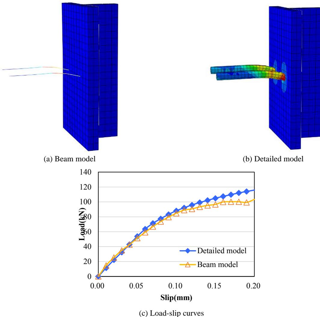
Fig. 13 Stresses and deformation distribution for different models
