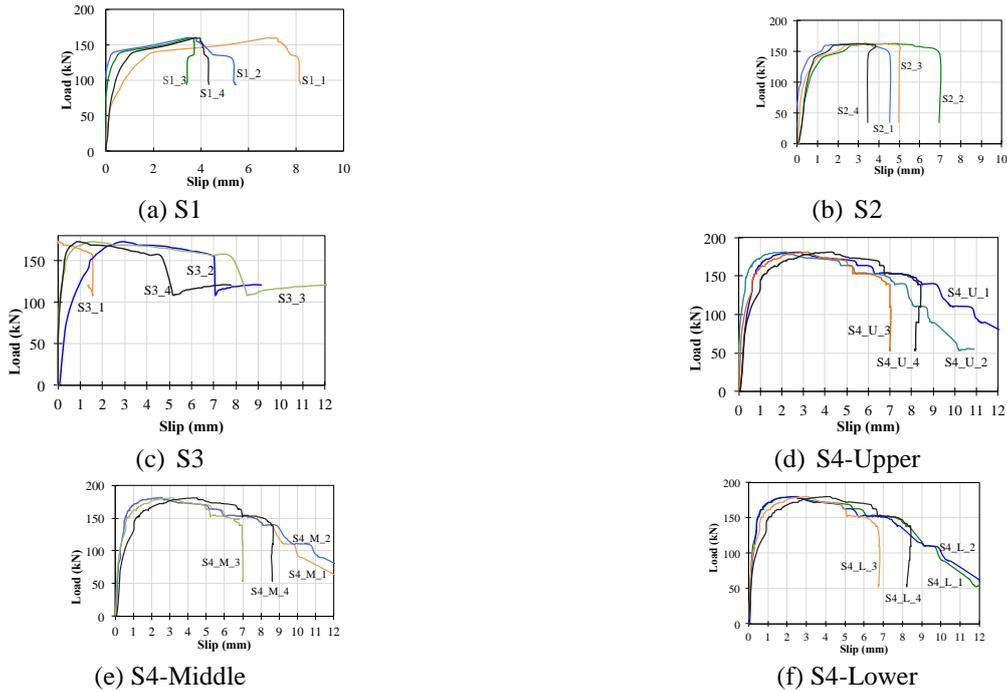
Fig. 6 Load-slip curves for all test specimens
