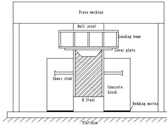
Fig. 4 Loading setup
