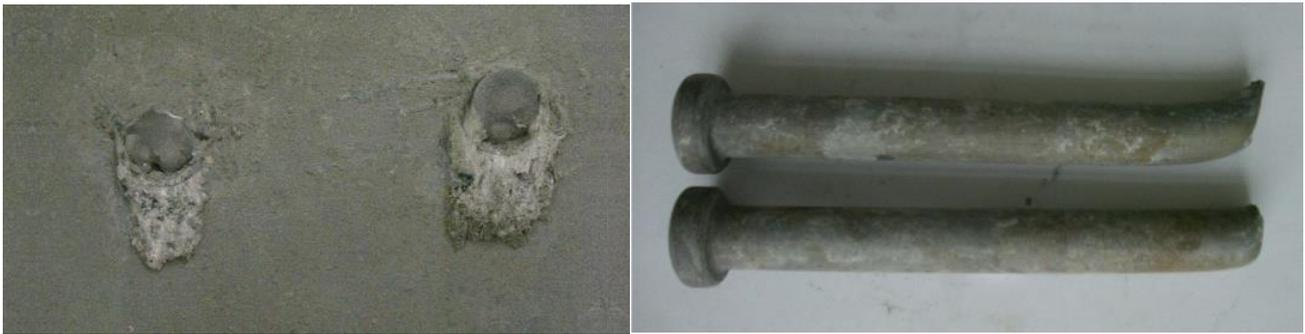
(a) Failure of shear studs
