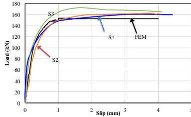
Fig. 9 Load-slip curve for test data and FE analysis results for S1 through S3
