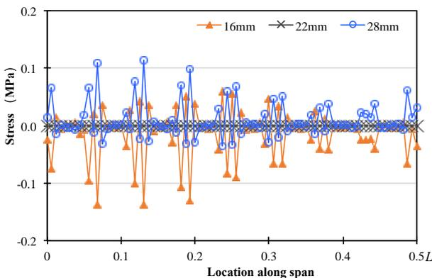
Fig. 18 Stress amplitude in bottom of concrete deck
