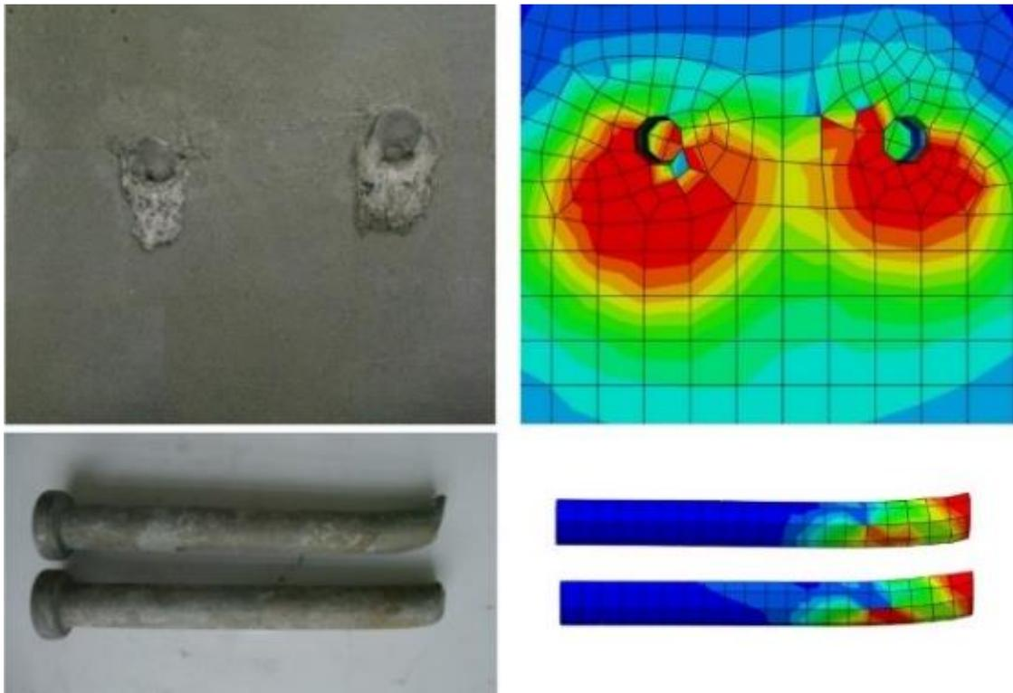
Fig. 12 Failure mechanisms of shear studs
