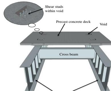
Fig. 1 Assembled twin-I girder with a precast concrete deck
