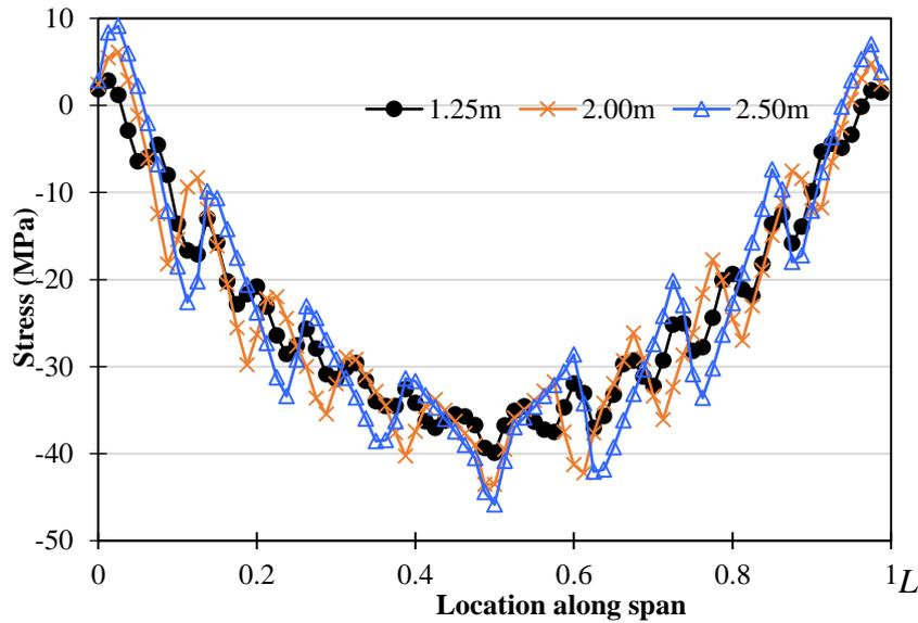
Fig. 17 Bottom flange stress in steel girders
