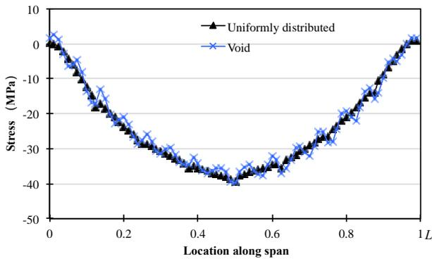
Fig. 15 Stresses distribution at top flange in steel girder
