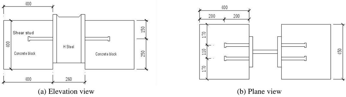
Fig. 2 View of test specimen S1 through S3 (unit: mm)
