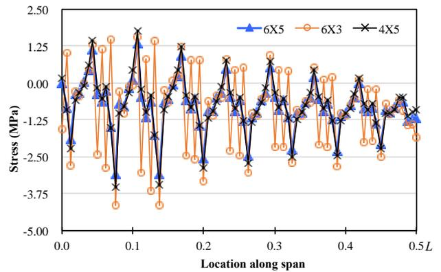
Fig. 19 Stress in concrete bottom surface for different longitudinal stud spacing
