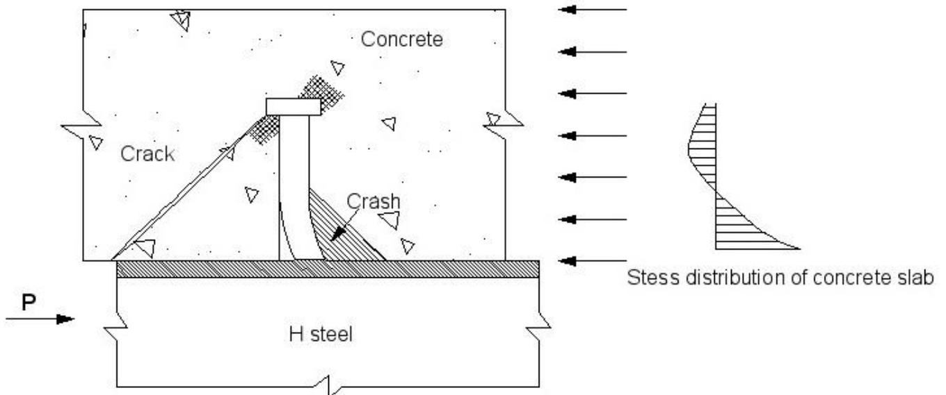
(b) Failure mechanisms between steel and concrete
