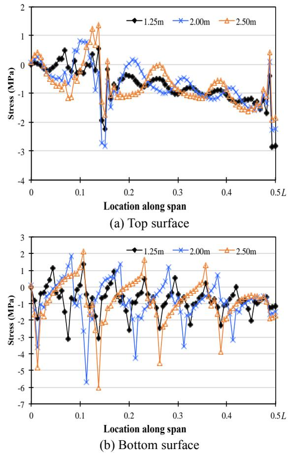
Fig. 16 Stress distribution in concrete deck
