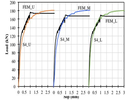
Fig. 10 Load-slip curve for test data and FE analysis results for S4
