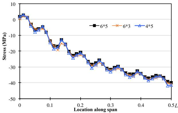
Fig. 20 Steel top flange stresses for different longitudinal stud spacing
