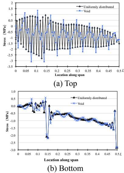
Fig. 14 Stresses distribution of concrete deck (half span)
