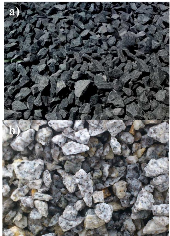
Fig. 4 The view of aggregates from igneous rocks: a) basalts, b) granites
