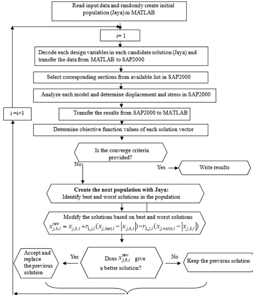
Fig. 1 Flowchart for the optimum design procedure of steel space frames
