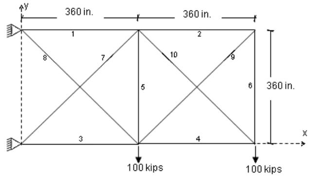
Fig. 3 10-bar plane truss
