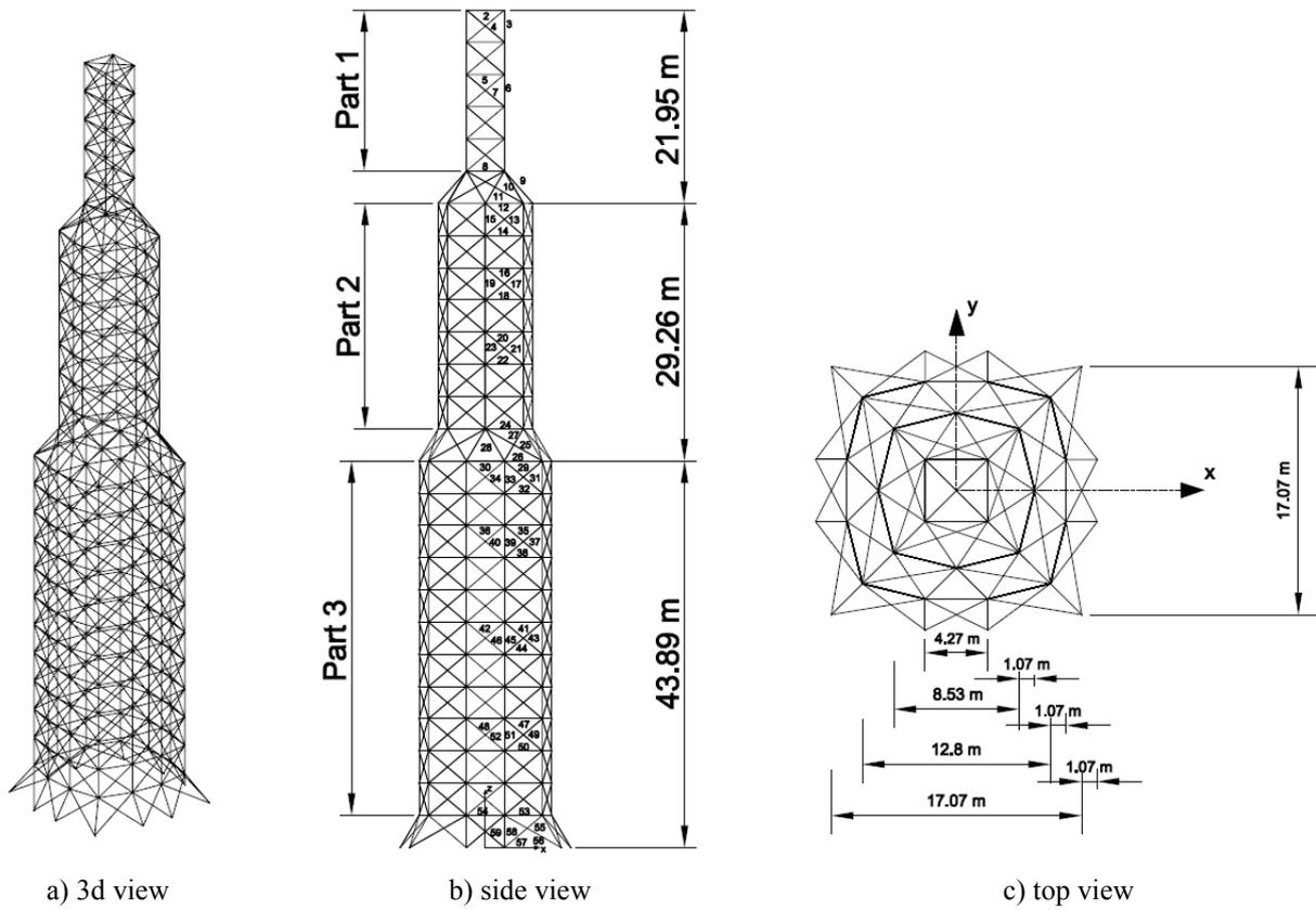
Fig. 7 942-Member space truss tower
