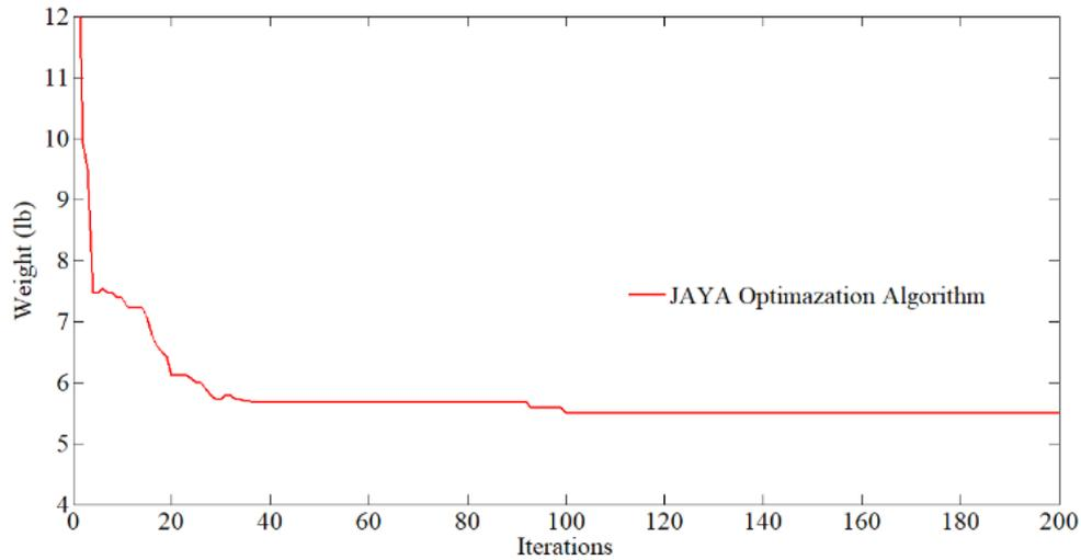
Fig. 4. Optimum design history of 10-bar plane truss
