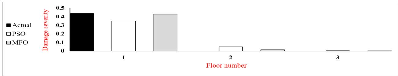
Fig. 16 Results of damage detection for LANL test structure – State #3
