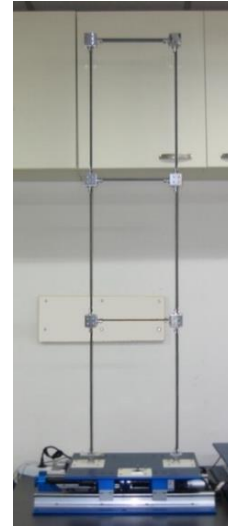
Fig. 7 Three-story shear building model for the experiment
