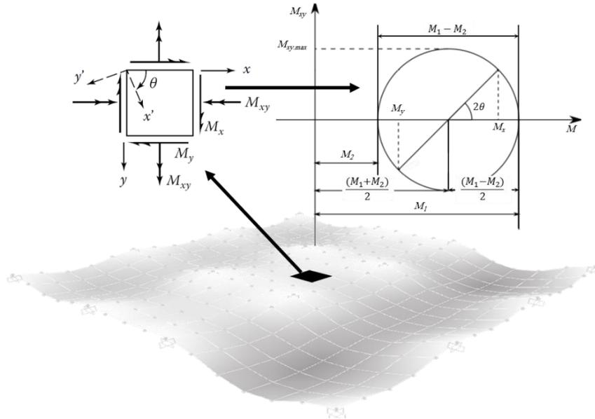
Fig. 1 Mohr circle concept illustration for an infinitesimal plate element
