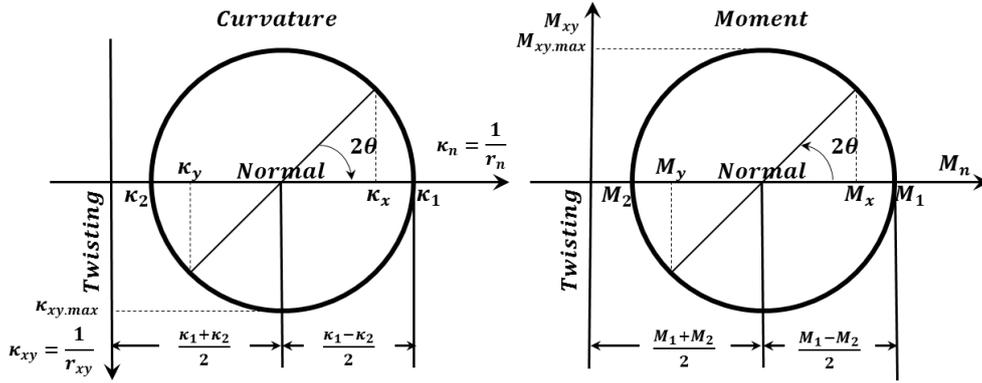
Fig. 2 Mohr circle representation and sign convention for curvature and moment
