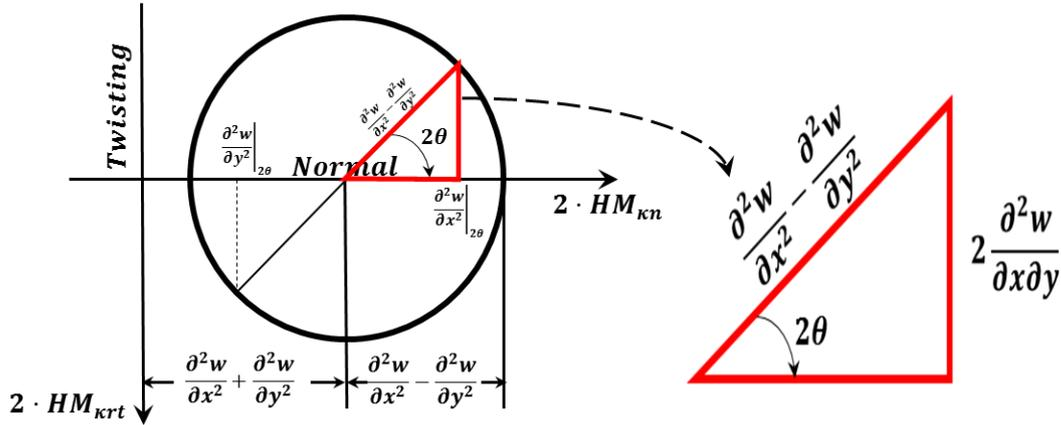
Fig. 6 The differential form of Mohr circle representation of curvature
