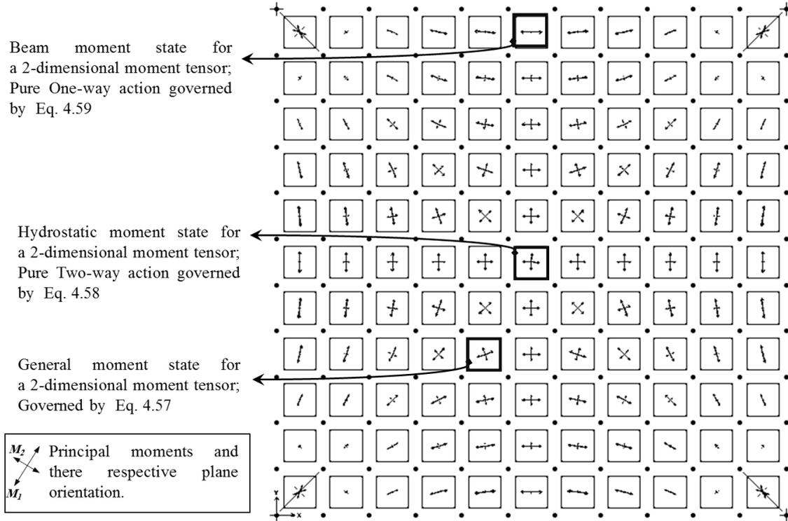
Fig. 5 Graphical illustration of the domain of applicability of various sub-terms of the introduced HM-Isotropic partial differential equation
