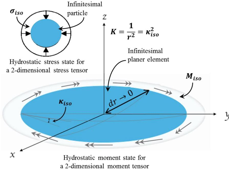
Fig. 3 Hydrostatic Moment and curvature representation in contrast to the hydrostatic stress representation
