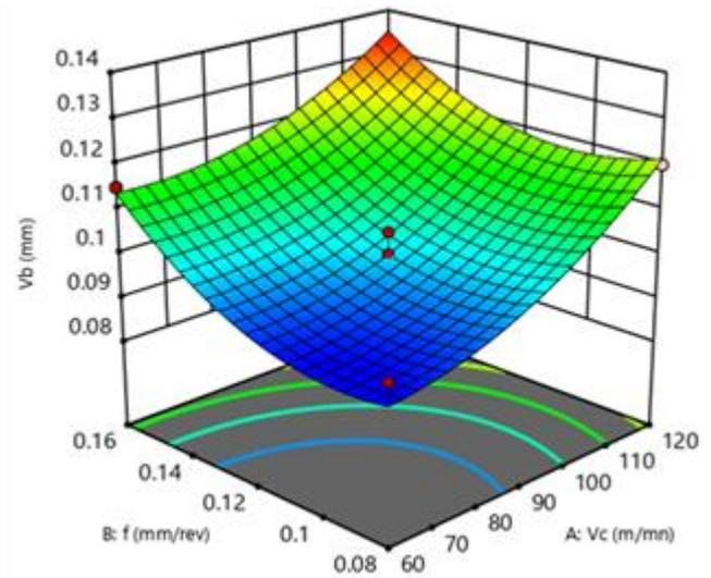
Fig. 8 3D surface graph for Interaction effects of feed and cutting speed on tool wear (VBmax)
