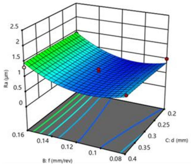
Fig. 4 3D surface graph for Interaction effects of feed rate and depth of cut on surface roughness
