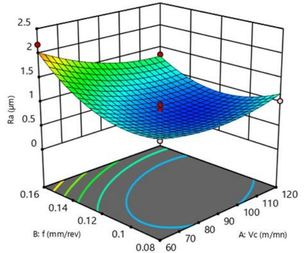
Fig. 2 3D surface graph for Interaction effects of feed rate and cutting speed on surface roughness
