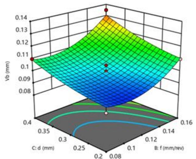
Fig. 10 3D surface graph for Interaction effects of feed and depth of cut on tool wear (VBmax)
