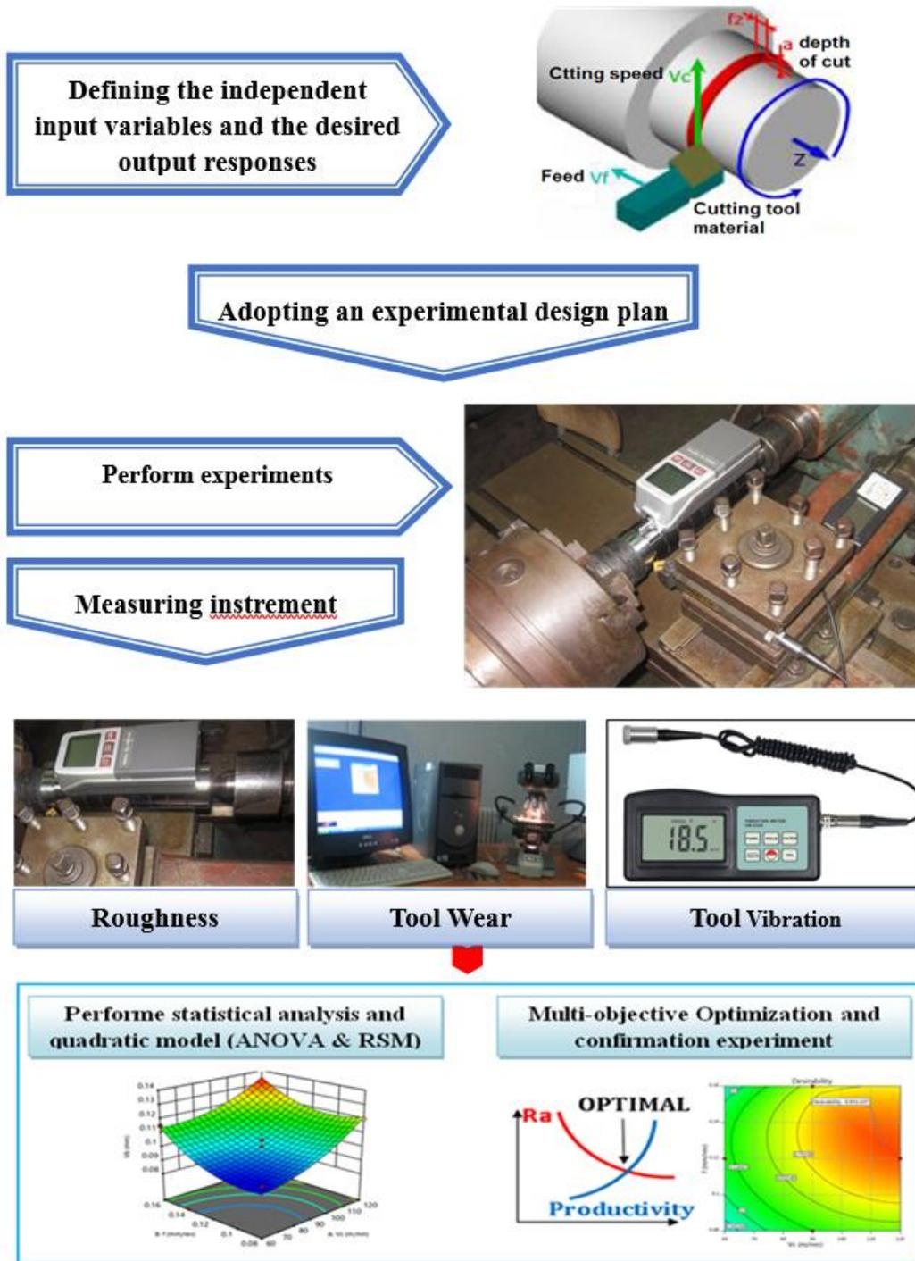
Fig. 1 Experimental design flowchart
