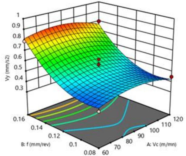
Fig. 5 3D surface graph for Interaction effects of feed rate and cutting speed on tool radial vibration ( $V_y$ )
