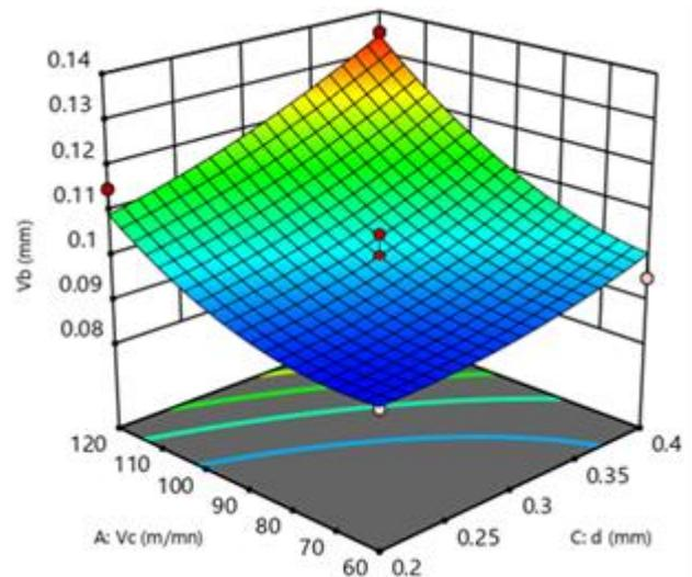
Fig. 9 3D surface graph for Interaction effects of depth of cut and cutting speed on tool wear (VBmax)
