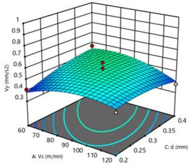
Fig. 6 3D surface graph for Interaction effects of cutting speed and depth of cut on tool radial vibration ( $V_y$ )
