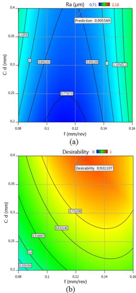
Fig. 14 Contour plot (a) for surface roughness and (b) for Desirability of multi-objective optimization, while (Vc) kept at the optimal value
