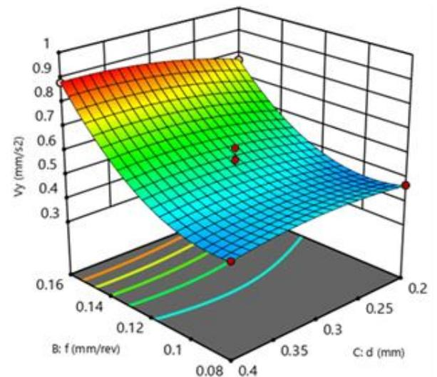
Fig. 7 3D surface graph for Interaction effects of feed and depth of cut on tool radial vibration ( $V_y$ )
