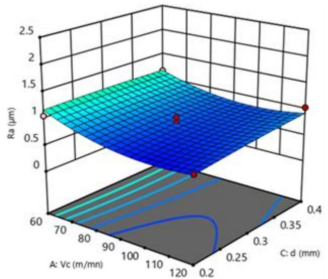
Fig. 3 3D surface graph for Interaction effects of depth of cut and cutting speed on surface roughness
