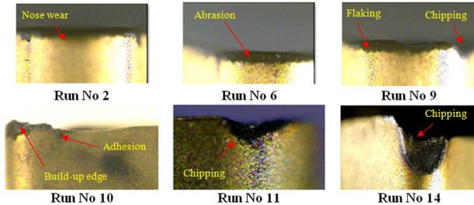
Fig. 11 Micro graphical of main wear mechanisms of coated carbide insert in hard turning [Run numbers according to table 2]
