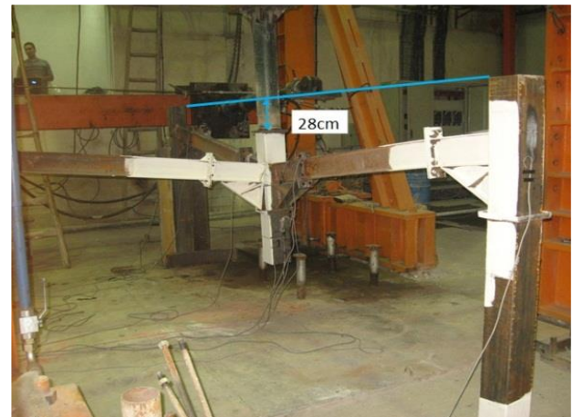
Fig. 18 Deformed shape of the frame with passive connections
