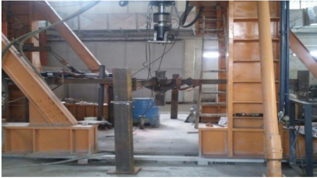
Fig. 16 Setup procedure of the frame with passive connections
