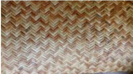
Fig. 1 Natural giant cane fiber mat after drying it for 12 hours at 70°C
