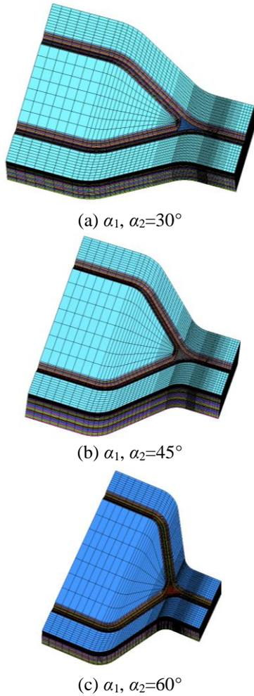
Fig. 3 Reservoir basin FEM model of different bifurcation angles
