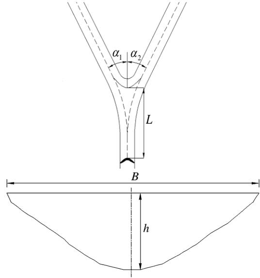
Fig. 2 Schematic diagram of bifurcation type reservoir basin
