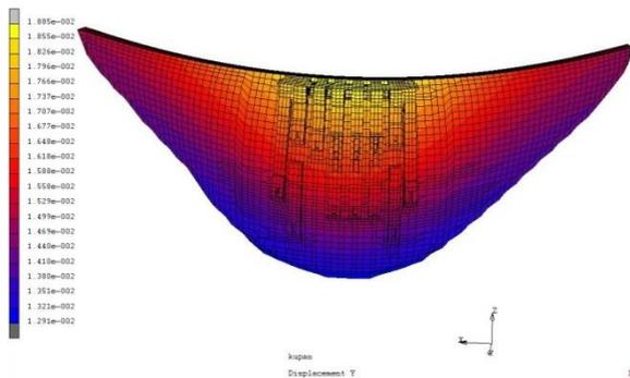
Fig. 17 Displacement of Xiaowan dam along the river at 1240 m water level
