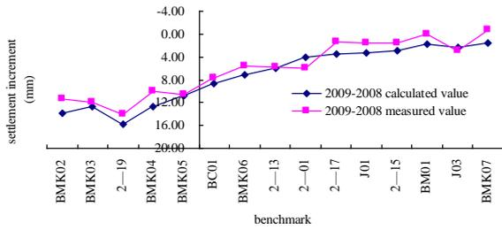
Fig. 15 Calculated and measured settlement increment of benchmarks on left bank between the year 2008 and 2009
