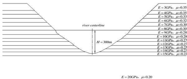
Fig. 5 Schematic diagram of geological stratification and mechanical parameters in reservoir basin model
