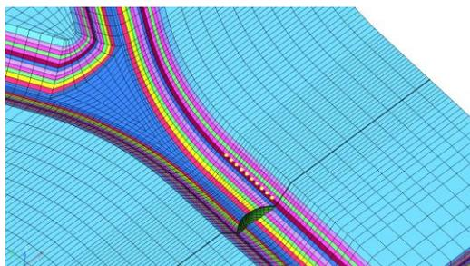
Fig. 4 Local details in FEM model of bifurcation type reservoir basin
