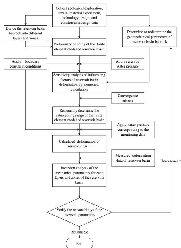
Fig. 1 Flowchart of inversion analysis for deformation modulus
