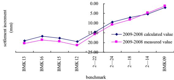
Fig. 16 Calculated and measured settlement increment of benchmarks on right bank between the year 2008 and 2009
