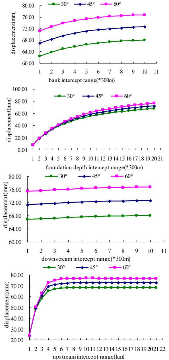
Fig. 6 Relationship between interception range of reservoir basin model and settlement of typical slope point for different bifurcation angles
