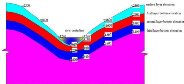
Fig. 12 Generalized graph of layers along vertical direction in zones I, II, III, V
