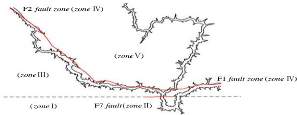
Fig. 11 Generalized geological zones along the horizontal direction of Xiaowan reservoir basin
