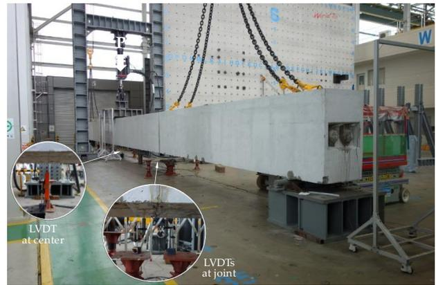
Fig. 11 Structural test and measurement of displacement for 30 m long HPSC girder
