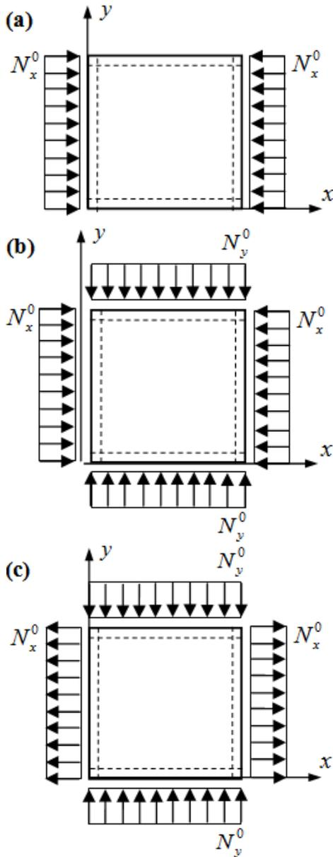
Fig. 2 The loading conditions of isotropic square plate for (a) uniaxial compression, (b) biaxial compression and (c) tension in the  $x$  direction and compression in the  $y$  direction
