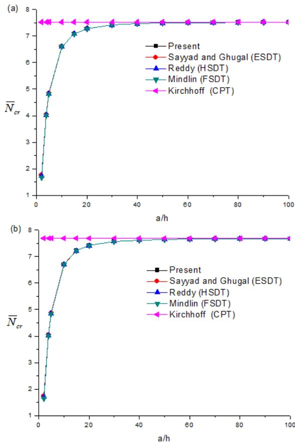
Fig. 5 The effect of side-to-thickness ratio on the critical buckling load of square plates subjected to tension in the  $x$ -direction and compression in the  $y$ -direction. (a) material 1 and (b) material 2
