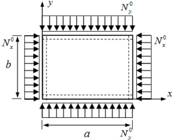
Fig. 1 Rectangular plate subjected to in-plane loads
