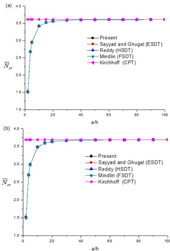
Fig. 3 The effect of side-to-thickness ratio on the critical buckling load of square plates subjected to uniaxial compression. (a) material 1 and (b) material 2
