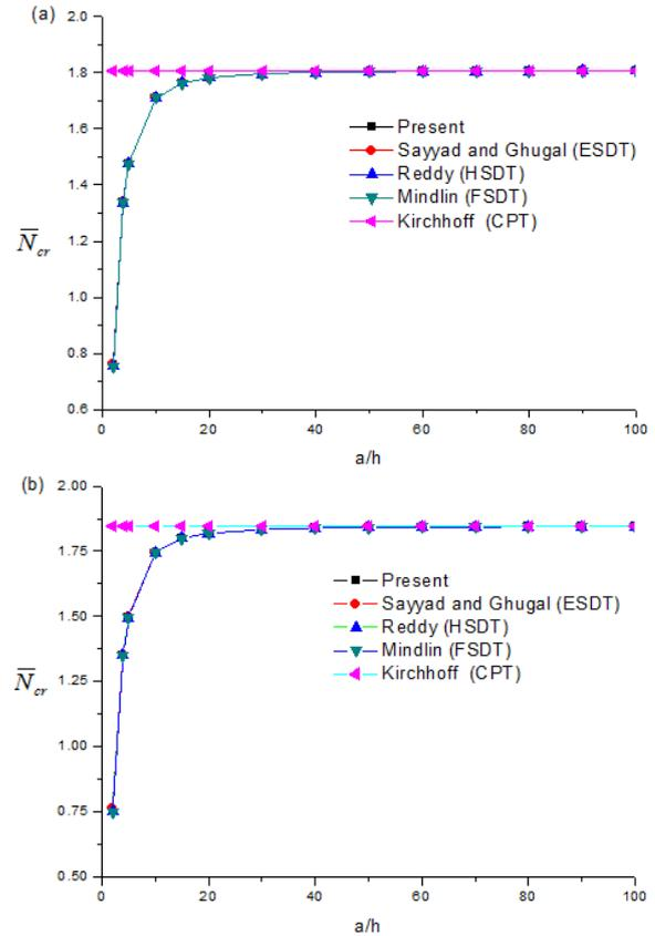
Fig. 4 The effect of side-to-thickness ratio on the critical buckling load of square plates subjected to biaxial compression. (a) material 1 and (b) material 2
